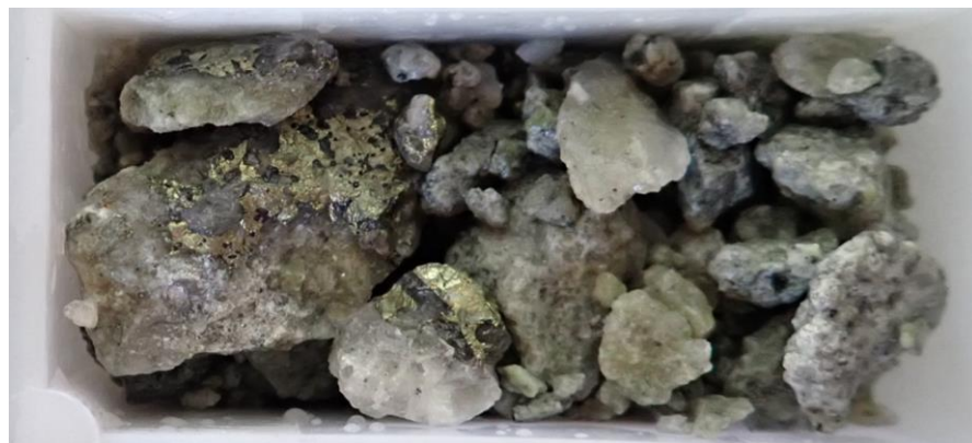
Figure 1 – Example of chalcopyrite mineralisation in drill hole BRURD002 (67 – 68m)
