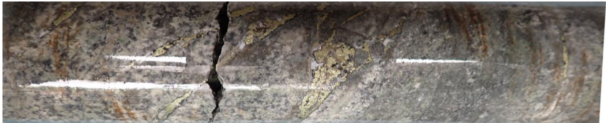
Figure 6 – Chalcopyrite-pyrite veins in strongly sericite-altered granodiorite in drill hole BRUDD002 (201.1 – 201.3m)
