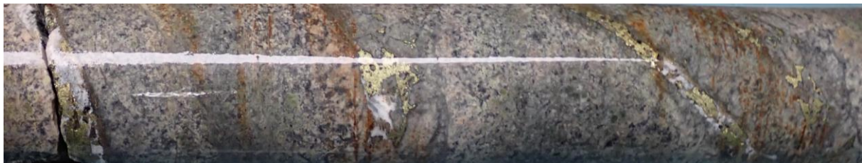
Figure 7 – Chalcopyrite-pyrite-quartz-carbonate veins in sericite-altered granodiorite in drill hole BRUDD002 (201.4 – 201.7m)
