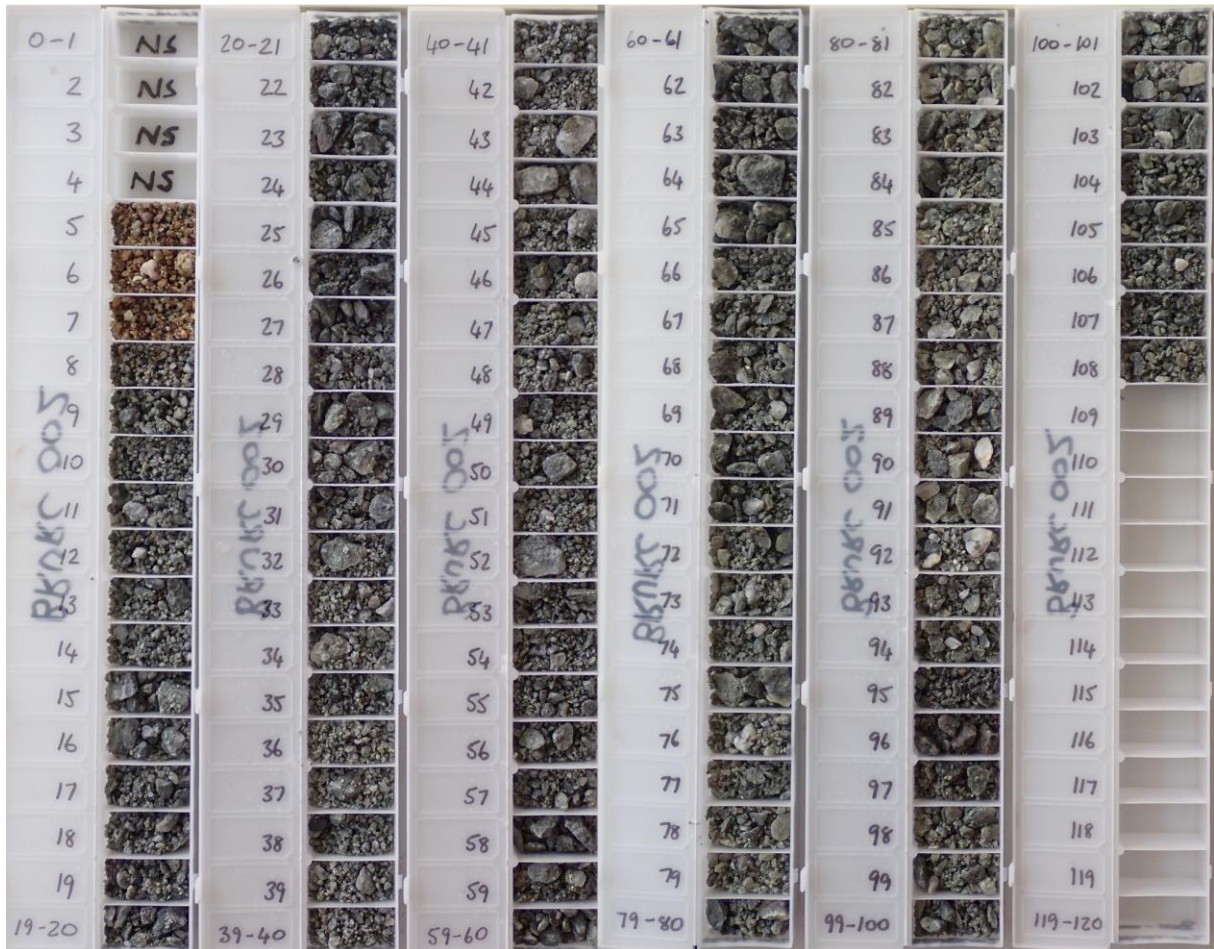
Figure 5 – Chip trays for BRURD002 pre-collar, exhibiting strong sericite-chlorite alteration and associated pyrite-chalcopyrite mineralisation
