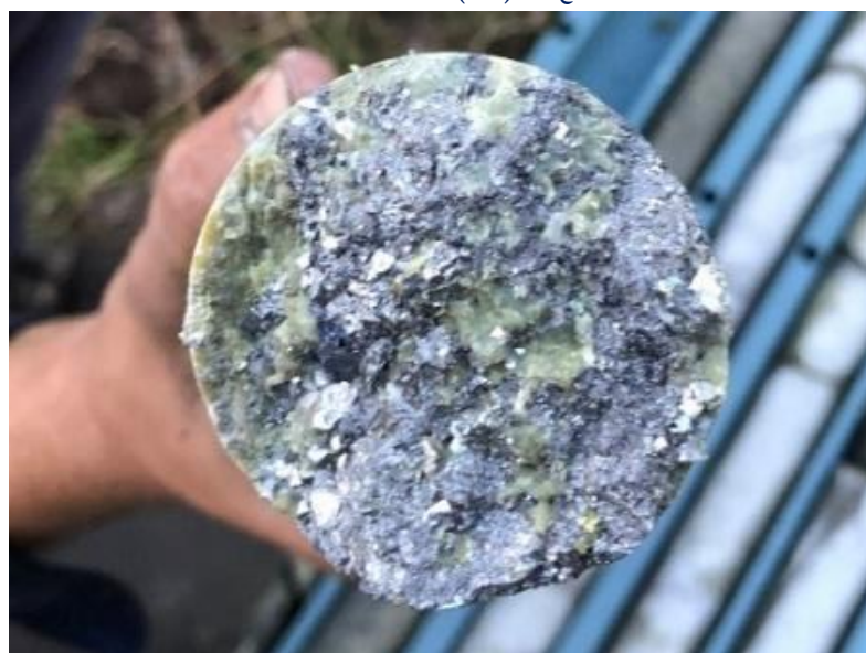
Photo 2: Coarse blebs of Glena (Pb) NQ 2 size drill core at Webbs Consol
