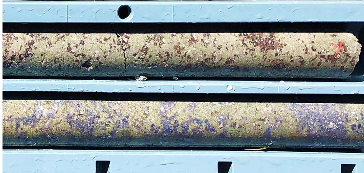
Photo 1: Sphalerite (Zn) and Galena (Pb) mineralisation in drill core (NQ2) from hole WCS023
