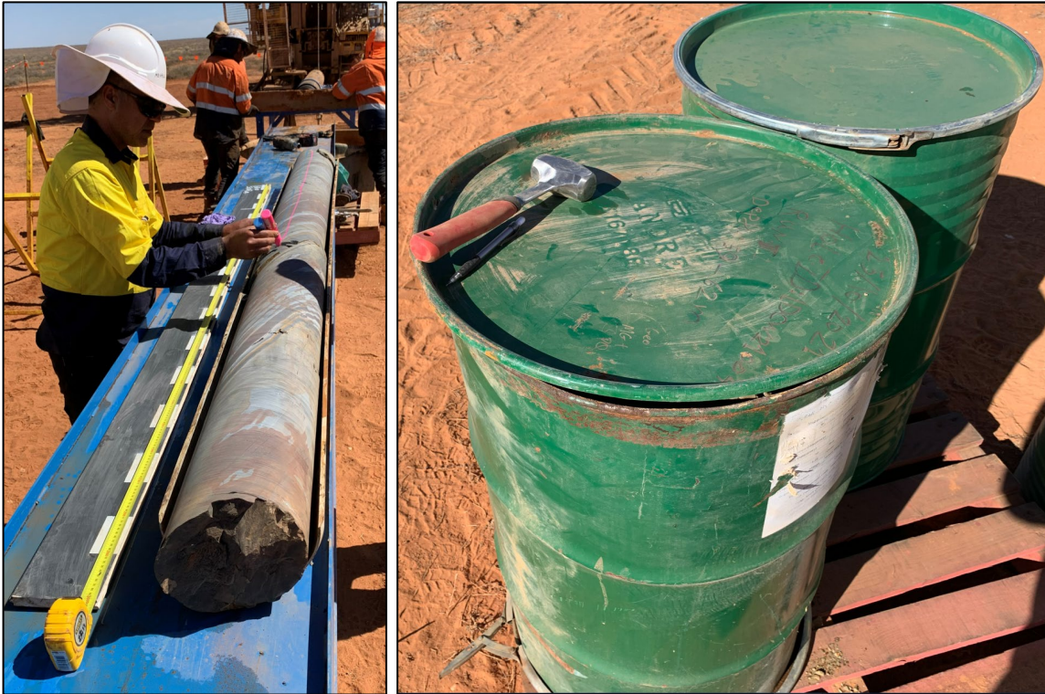
Figure 6: Large diameter (8" = 200mm) corehole LDCW21004 for comminution testing and 400L drum for storage and transport.
