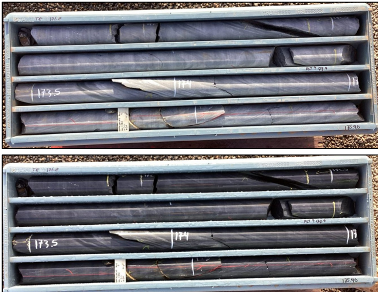
Figure 5: Photo of HQ3 geotechnical core: GPFO22047 171.80-175.90m (top = dry, bottom = wet). The core plug on the bottom flute denotes where a sample was taken from.
