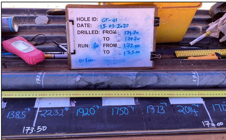
Figure 8a: Marked up core for lithology logging on the core table at the rig site (blue chalk numbers are magnetic susceptibility readings). The CormaGeo RT-1 Magnetic Susceptibility Meters used to take these measurements is at the top left (pink).
