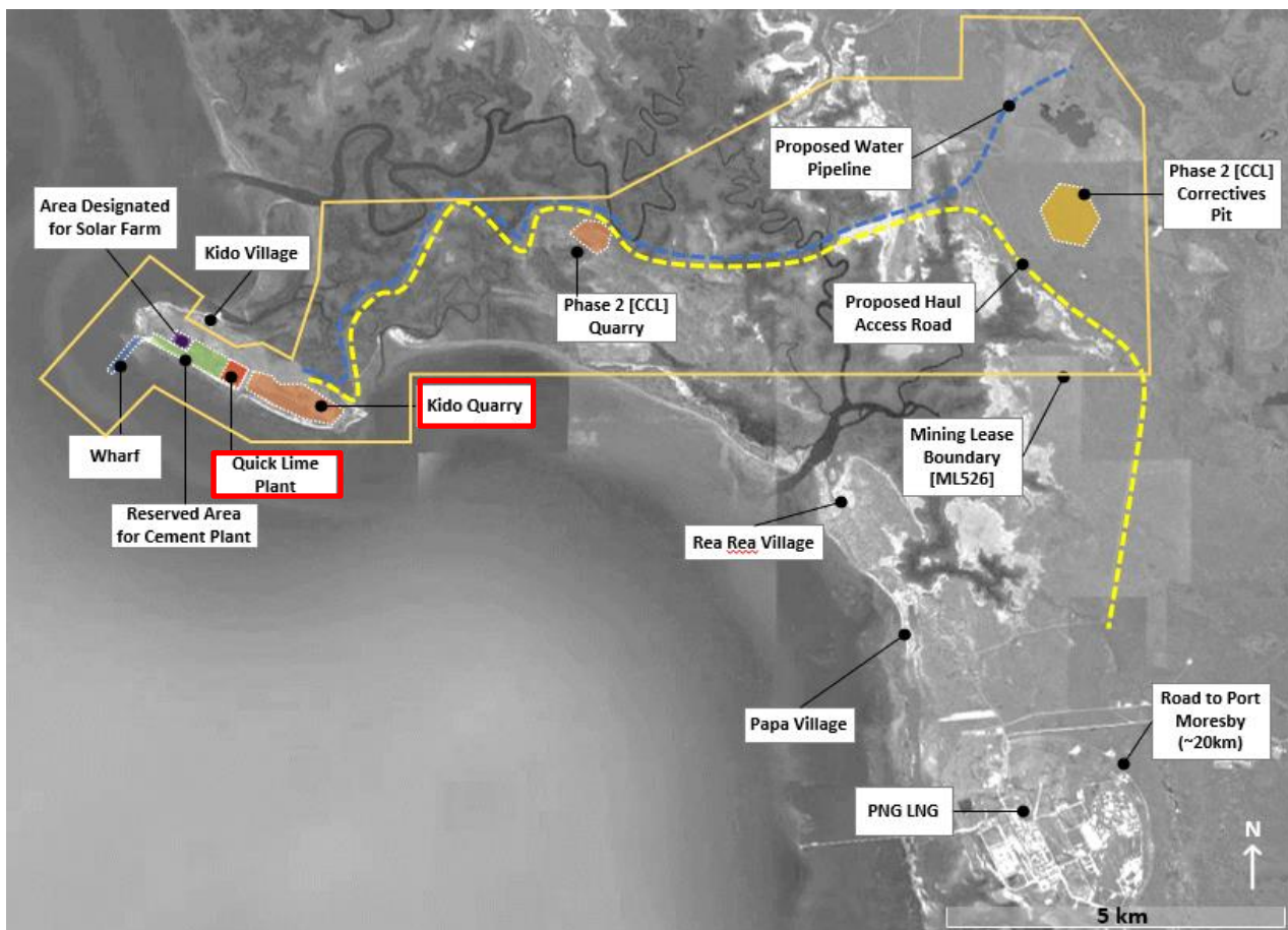
Figure 10: CCL Project general arrangement within ML 526 (orange polygon) and Kido quarry and lime plant in red outline
