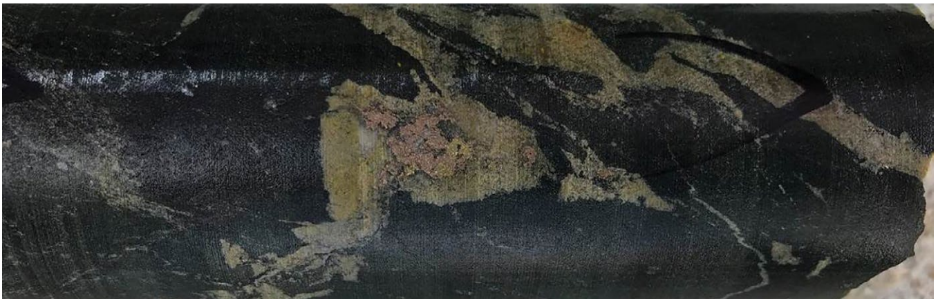
Figure 11: LBSDD001 – 94m – fine-grained melanogabbro with an irregular syn-genetic feldspar tremolite vein with blebby magmatic sulphide. Field of view from top to bottom ~ 47mm.
