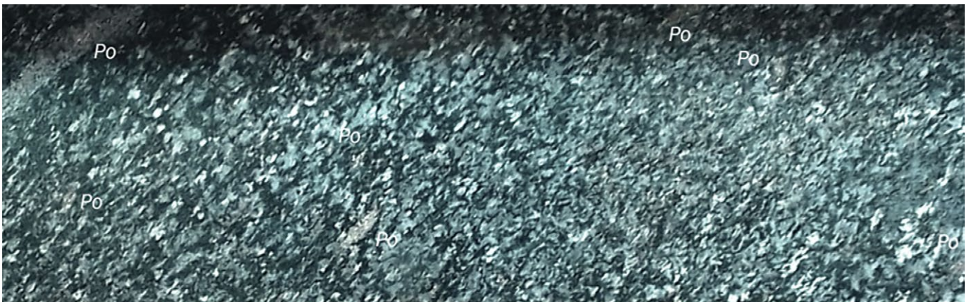
Figure 6: LBNDD002 – 355.50m – blebby magmatic sulphide mineralisation hosted in a varitextured, contaminated gabbro. Field of view from top to bottom ~36mm.
