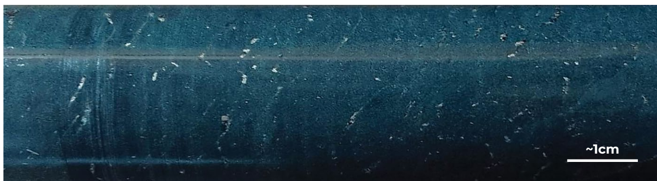
Figure 9: MTCDD003 – 125.00m – Disseminated magmatic sulphides within a very fine-grained wehrlite (chill margin).
