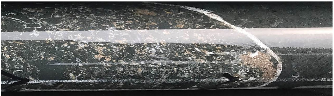
Figure 12: LBSDD002 – 208m – Mafic breccia in contact with a fine to medium grained clinopyroxenite with strongly disseminated to matrix magmatic sulphide on the contact. Field of view from top to bottom ~ 36mm.
