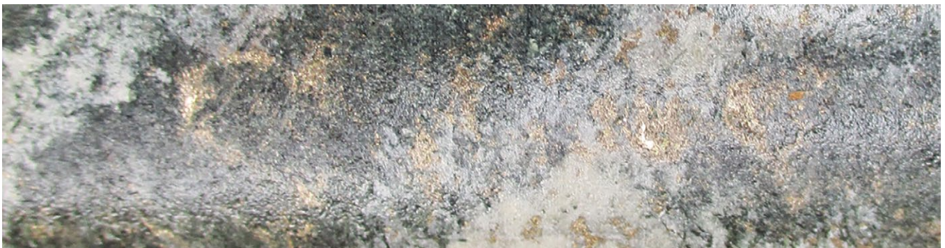
Figure 5: LBNDD001 –246.00m – blebby magmatic sulphide mineralisation associated with a feldspar vein in a medium to coarse grained granular clinopyroxenite. Field of view from top to bottom ~30mm.
