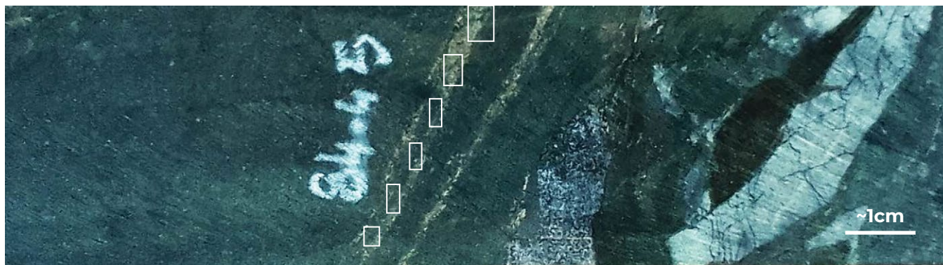
Figure 7: MTCDD001 – 84.45m – fine grained poikilitic wehrlite with vein magmatic sulphide concentrated along the micro-sill margin (dotted line) – in contact with a magmatic breccia.
