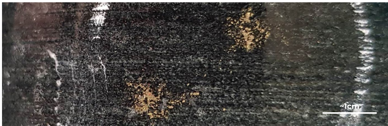
Figure 8: MTCDD002 – 54.85m – blebby magmatic sulphide within a fine-grained poikilitic wehrlite.
