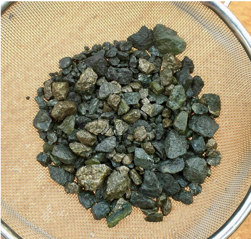
Figure 18: RC chips from REYRC002 79-80m showing net-textured / brecciated Ni-Cu sulphides (~15-20%) comprised of pyrrhotite, chalcopyrite and pentlandite.
