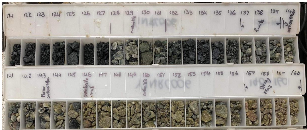
Figure 10: Chip tray from YINRC006 showing dark fenitic alteration grading into two mineralised fresh ironstones (ferrocarnatite) from 127-131m and 139m-160m.
