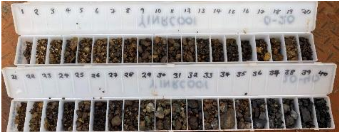
Figure 9: Chip tray from YINRC001 showing mineralised oxidized ironstone from 1-34m and grading into dark fenitic alteration.
