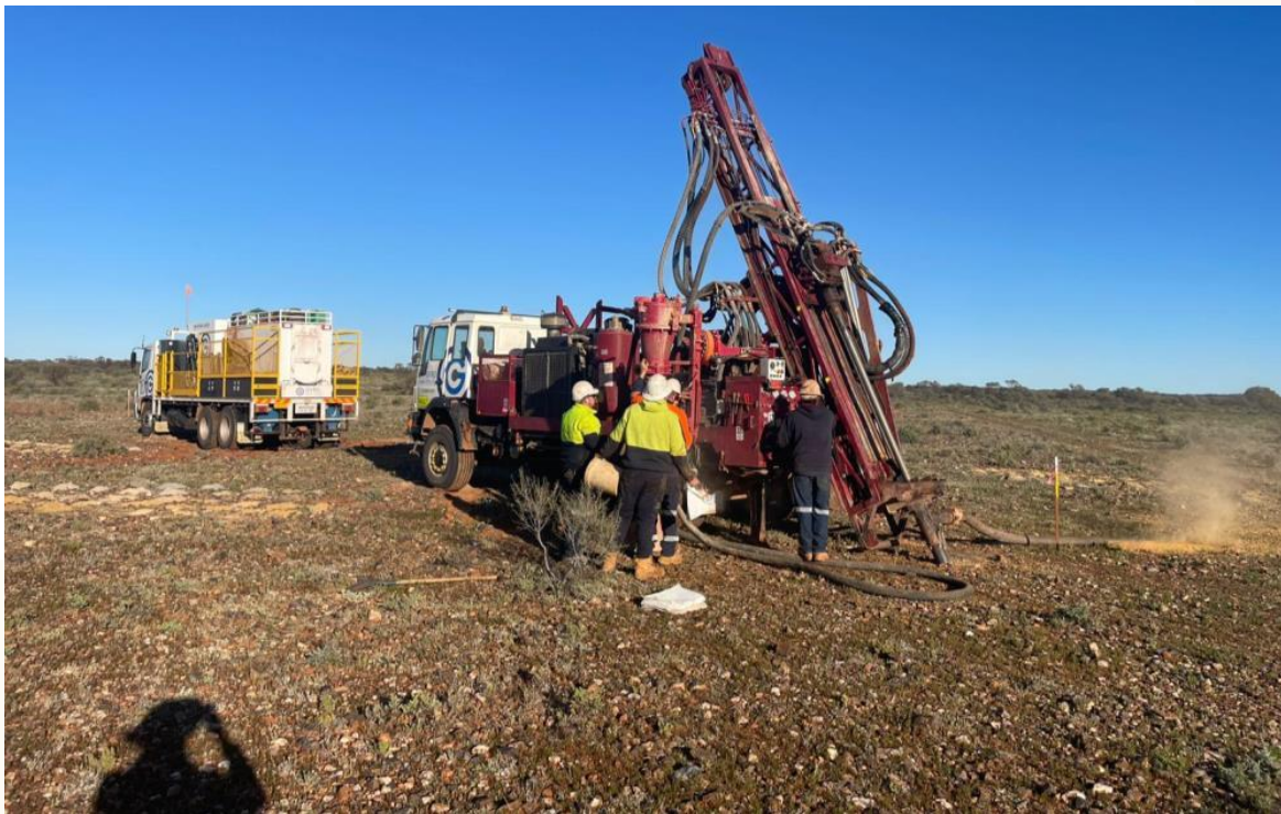
Figure 7: Aircore Drilling Rig at Everlong Prospect of the Austin Gold Project
