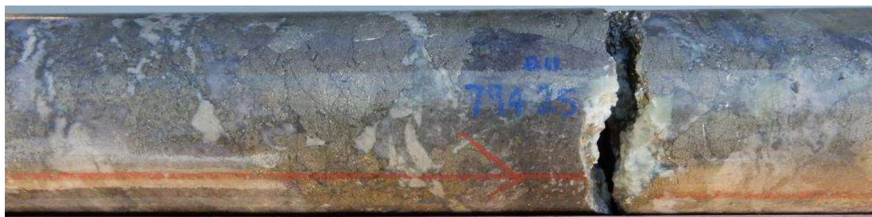
Fig 15 HQ Core photo hole 22CAEDD0011, 794.25m , semi-massive sulphide infill of quartz, pyrite, chalcopyrite, within sulphidic breccia. Interval 794m to 795m assays 1m @ 1.68% Cu,9.83 g/t Au, 60.9 g/t Ag, 17.44% S
