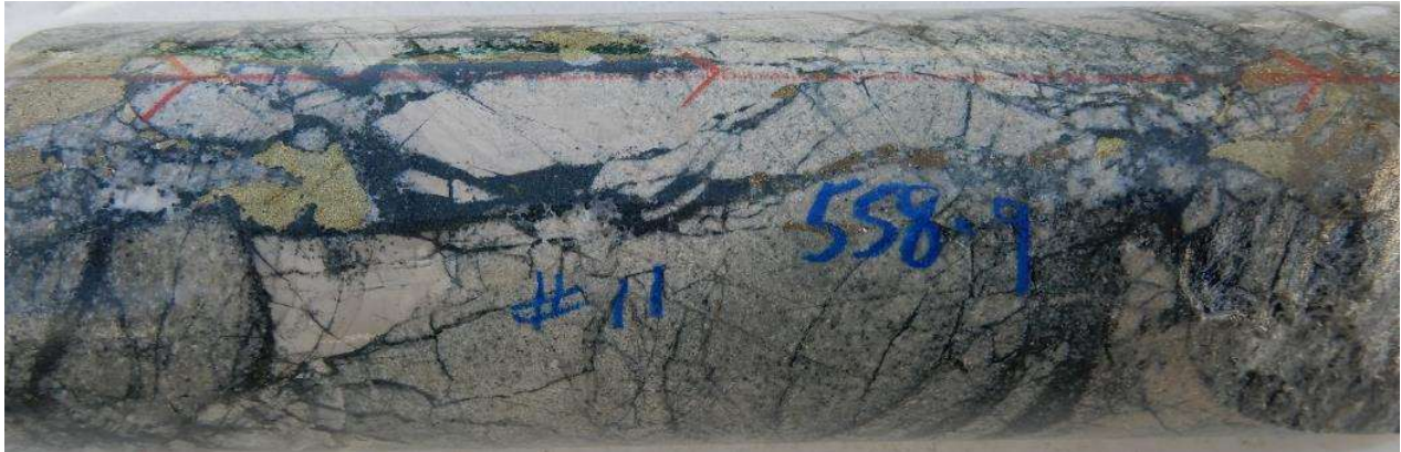
Fig 8. HQ Core photo hole 22CAEDD0011, 558.1m , chalcopyrite -pyrite , chlorite quartz infill in breccia dominated by hornfelsed siltstone/sandstone clasts. Interval 558m-559m assays 1m @ 2.09% Cu,0.38 g/t Au, 15.5 g/t Ag, 8.65 % S
