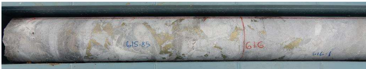
Fig 11 HQ Core photo hole 22CAEDD0011, 616m , chalcopyrite -pyrite , calcite infill in breccia dominated by hornfelsed siltstone/sandstone clasts. Primary zone 615m-617m assays 2m @ 0.77% Cu,0.18 g/t Au, 10.3 g/t Ag, 4.14 % S
