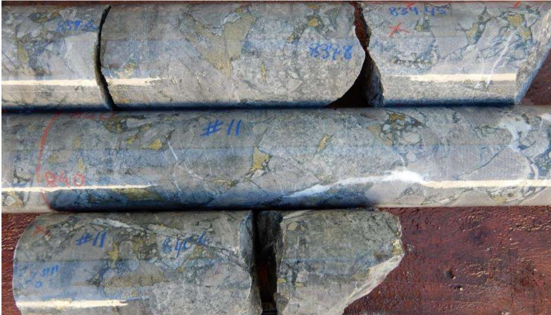
Fig 19 HQ Core photo hole 22CAEDD0011, Selected samples 839.8m,840m,840.4m , Polymict breccia with subrounded to subangular clasts hornfels, altered diorite , porphyry prominent infill of chalcopyrite -pyrite , carbonate, quartz ,chlorite. Interval 839m to 841m assays 2m @ 0.69% Cu,0.14 g/t Au, 17.9 g/t Ag, 2.19% S
