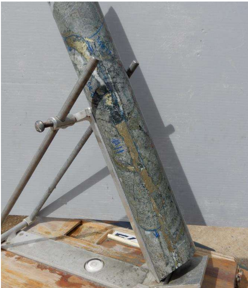
Fig 9 HQ Core photo hole 22CAEDD0011, 558.2m , chalcopyrite -pyrite , chlorite quartz infill in structure running through breccia dominated by hornfelsed sandstone clasts. Primary zone 558m-559m assays 1m @ 2.09% Cu,0.38 g/t Au, 15.5 g/t Ag, 8.65 % S
