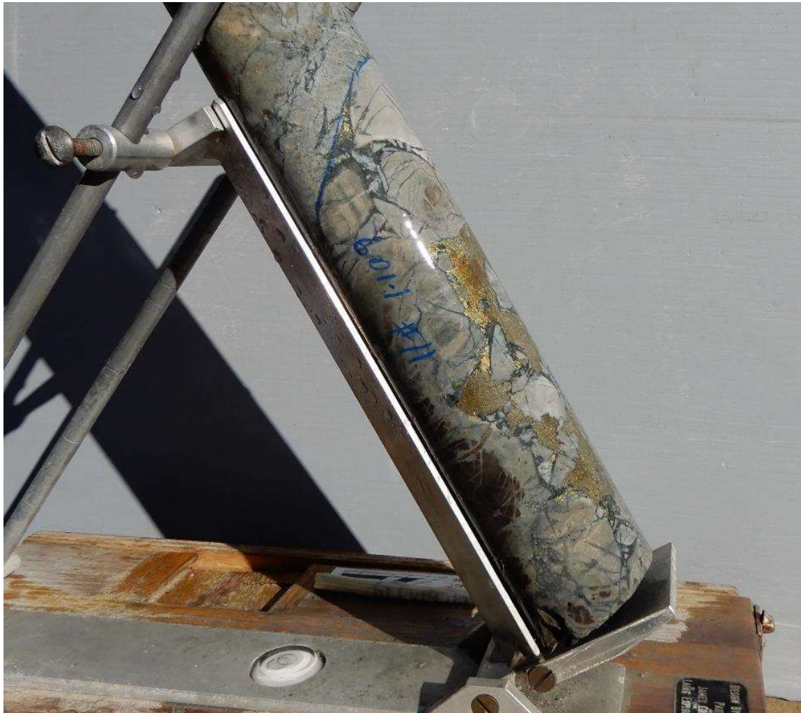
Fig 10 HQ Core photo hole 22CAEDD0011, 601.1m , -pyrite , chalcopyrite chlorite infill in breccia dominated by hornfelsed sandstone clasts. Primary zone 601m-602m assays 1m @ 0.1% Cu,0.02 g/t Au, 1.3 g/t Ag, 0.7 % S
