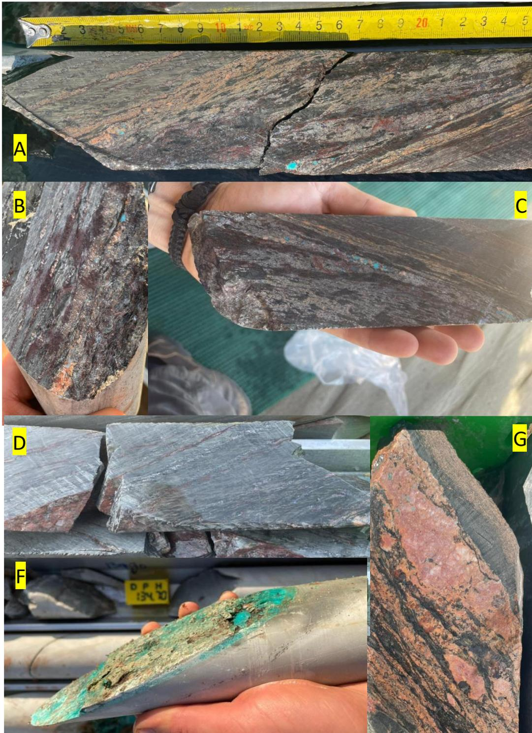
Figure 1. Examples of: chalcocite mineralisation (A - D) which appears as a silver-grey metallic mineral in the photos, (E) malachite and chrysocolla mineralisation on fracture planes in the upper mineralised portion and (G) potassic alteration with chlorite and chalcocite in veins near the contact with the Ngwako Pan Formation.
