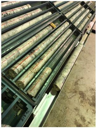
Figure 4: Processing pegmatite core at LPM Darwin Facility
