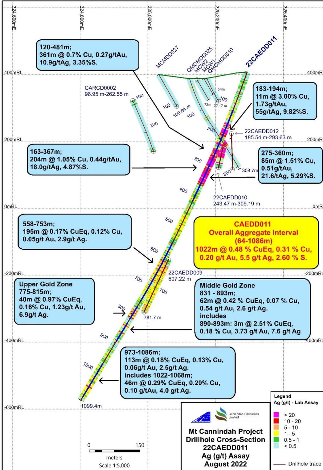
Fig 7. Mt Cannindah mine area east-west cross section CAE hole 11 looking north, with Ag lab assay results plotted down hole, significant intersections annotated. All Assays reported for CAE hole # 11 from 0m to 1099.4m
