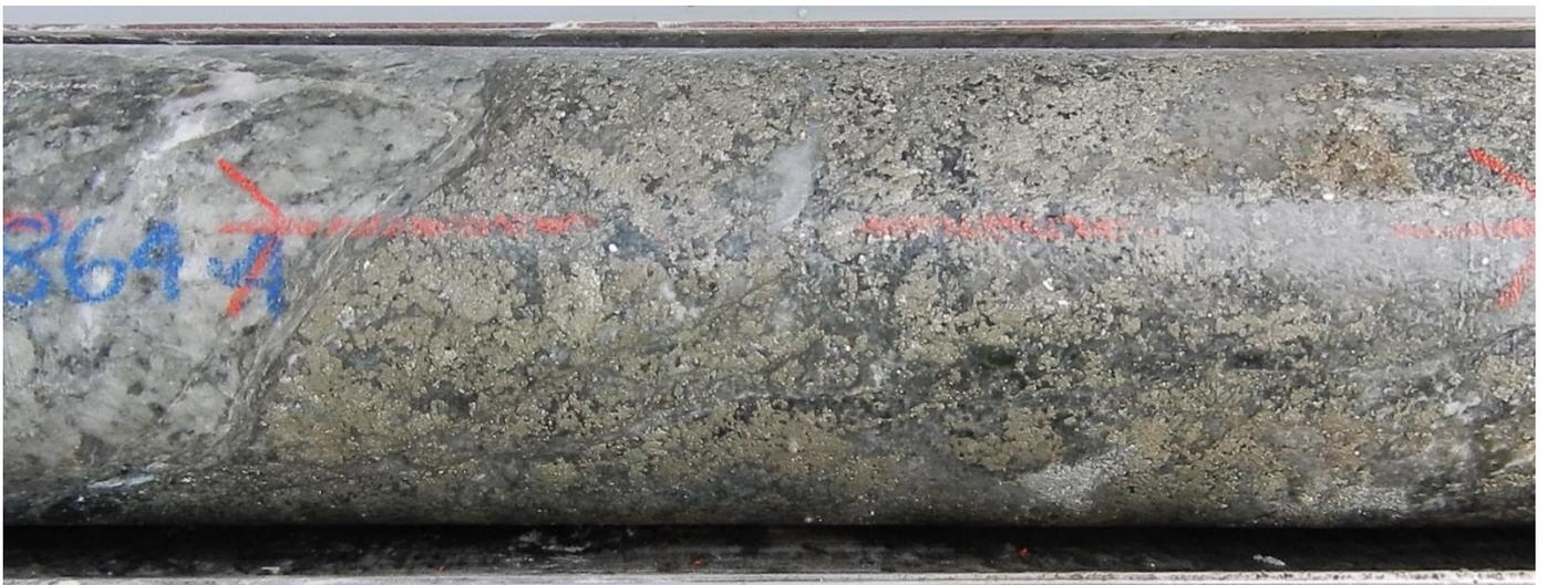
Fig 8. NQ Core photos hole 22CAEDD0011, 864.5m , polymict clast supported breccia with clasts of hornfels and diorite, minor altered rock-flour matrix. Strong pyrite – silica-carbonate alteration and infill. Interval 864m-865m assays 1m @ **7.73 g/t Au 0.14% Cu, , 13.8 g/t Ag, 7.6 % S**
