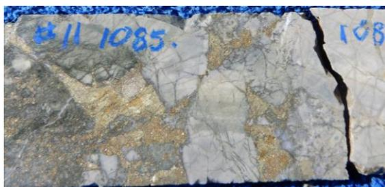
Deepest copper zone intersected to date at 1085m : chalcopyrite-pyrite infill in clast supported breccia with altered rock flour matrix.
