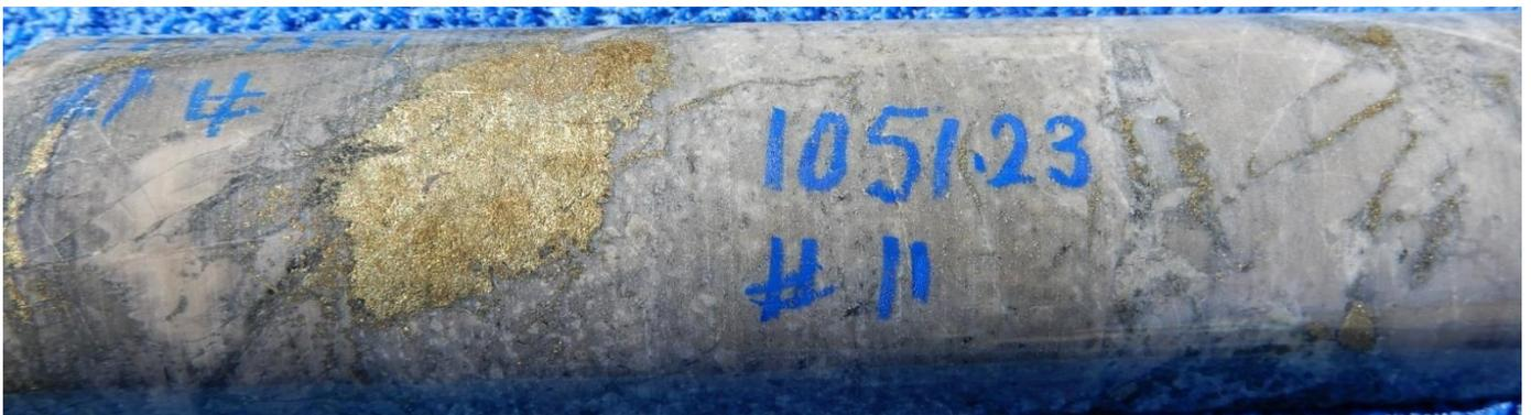
Fig 16. NQ Core photos hole 22CAEDD0011, 1051.23m Chalcopyrite, pyrite, quartz, infill , some sulphide veins, within clast supported breccia ,dominated by hornfels clasts with some diorite. Interval 1051m-1052m assays 1m @ **0.34 g/t Au 0.72% Cu, , 14.2 g/t Ag, 5.83 % S.**
