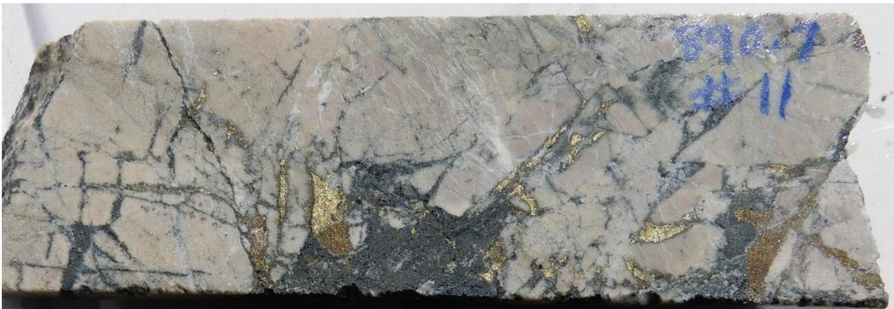
Fig 11. NQ Core photos hole 22CAEDD0011, 890.7m ,Sericitic altered ,clast supported breccia with chlorite -rock flour matrix , pyrite -chalcopyrite chlorite infill. Interval 890m-891m assays 1m @ **10.0 g/t Au 0.46% Cu , , 17.5 g/t Ag, 2.21 % S**
