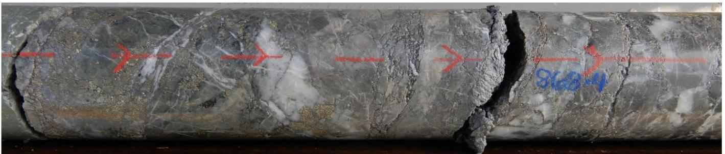
Fig 9. NQ Core photos hole 22CAEDD0011, 868.4m , Quartz sericite pyrite infill of shear/fault zone within clast supported breccia. Interval 868m-869m assays 1m @ **2.58 g/t Au 0.06% Cu, , 5.0 g/t Ag, 2.8 % S**
