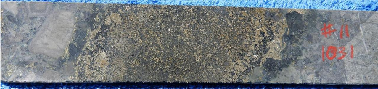
Fig 13. NQ Core photos hole 22CAEDD0011, 1030.9m ,Sericitic altered ,clast supported breccia , pyrite, chalcopryite, chlorite, quartz infill. Semi-massive sulphide section of metre. Interval 1030m-1031m assays 1m @ **0.32 g/t Au 0.73% Cu, , 15 g/t Ag, 5.41 % S.**
