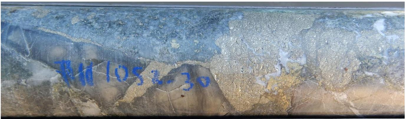
Fig 17. NQ Core photos hole 22CAEDD0011, 1052.3m Chalcopyrite,pyrite,quartz,calcite chlorite infill , , within clast supported breccia ,dominated by hornfels clasts with chloritized rock flour matrix. Interval 1052m-1053m assays 1m @ **0.47 g/t Au 0.99% Cu, , 22.5 g/t Ag, 6.24 % S.**
