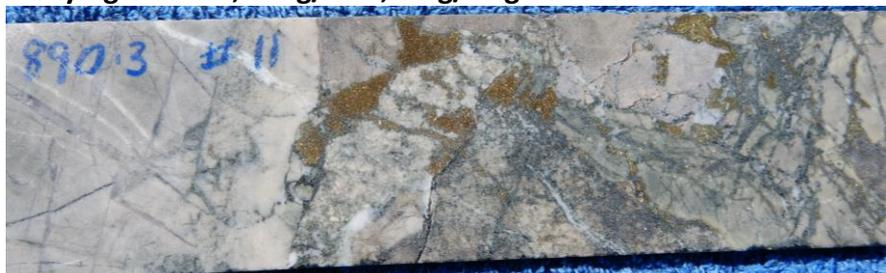
Chlorite matrix clast supported breccia with pyrite chalcopyrite infill 890.3m.
