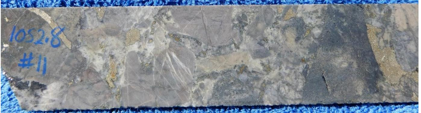
Fig 18 NQ Core photos hole 22CAEDD0011, 1052.8m Chalcopyrite, pyrite, quartz, calcite chlorite infill , within clast supported breccia ,dominated by hornfels clasts with chloritized rock flour matrix. Polymict clasts some stockwork veined. Interval 1052m-1053m assays 1m @ **0.47 g/t Au 0.99% Cu, , 22.5 g/t Ag, 6.24 % S.**
