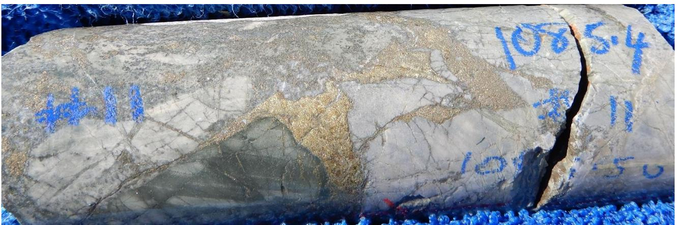
Fig 19 NQ Core photos hole 22CAEDD0011, 1085.4m Chalcopyrite, pyrite, chlorite, quartz, calcite infill, within clast supported breccia ,dominated by hornfels clasts with chloritized rock flour matrix. Deepest copper zone intersected. Interval 1085m-1086m assays 1m @ **0.33 g/t Au 0.49% Cu, ,7.5 g/t Ag, 2.91 % S.**
