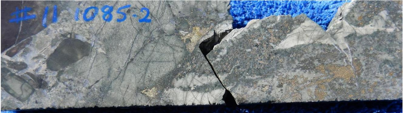
Fig 20 NQ Core photos hole 22CAEDD0011, 1085.2m chlorite quartz, calcite , pyrite ,chalcopyrite, infill , within clast supported breccia ,dominated by hornfels clasts with chloritized rock flour matrix. Hornfels clasts cut by stockwork of vein fracture network. Deepest copper zone intersected to date at Mt Cannindah breccia. Interval 1085m-1086m assays 1m @ **0.33 g/t Au 0.49% Cu, ,7.5 g/t Ag, 2.91 % S.**
