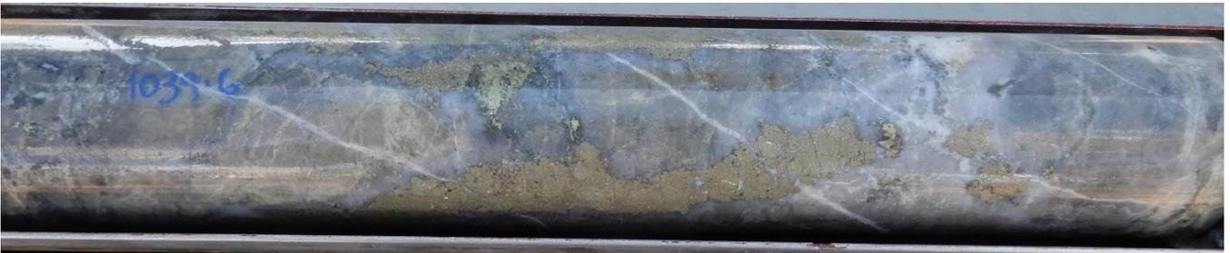
Fig 14. NQ Core photos hole 22CAEDD0011, 1039.6m ,Sericitic altered ,clast supported breccia , quartz,pyrite, chalcopryite infill. Interval 1039m-1040m assays 1m @ **0.27 g/t Au 0.34% Cu, , 6.5 g/t Ag, 3.36 % S.**
