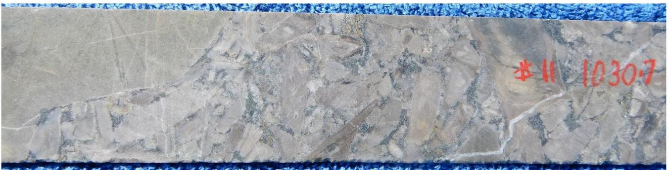
Fig 12. NQ Core photos hole 22CAEDD0011, 1030.7m ,Sericitic altered ,clast supported breccia , pyrite chlorite infill. Low sulphide section of metre. Interval 1030m-1031m assays 1m @ **0.32 g/t Au 0.73% Cu , , 15 g/t Ag, 5.41 % S.**
