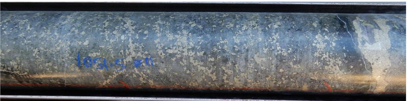
Fig 15. NQ Core photos hole 22CAEDD0011, 1051.5m Pyrite, quartz, chlorite, chalcopryite infill within section of, clast supported breccia , Interval 1051m-1052m assays 1m @ **0.34 g/t Au 0.72% Cu, , 14.2 g/t Ag, 5.83 % S.**
