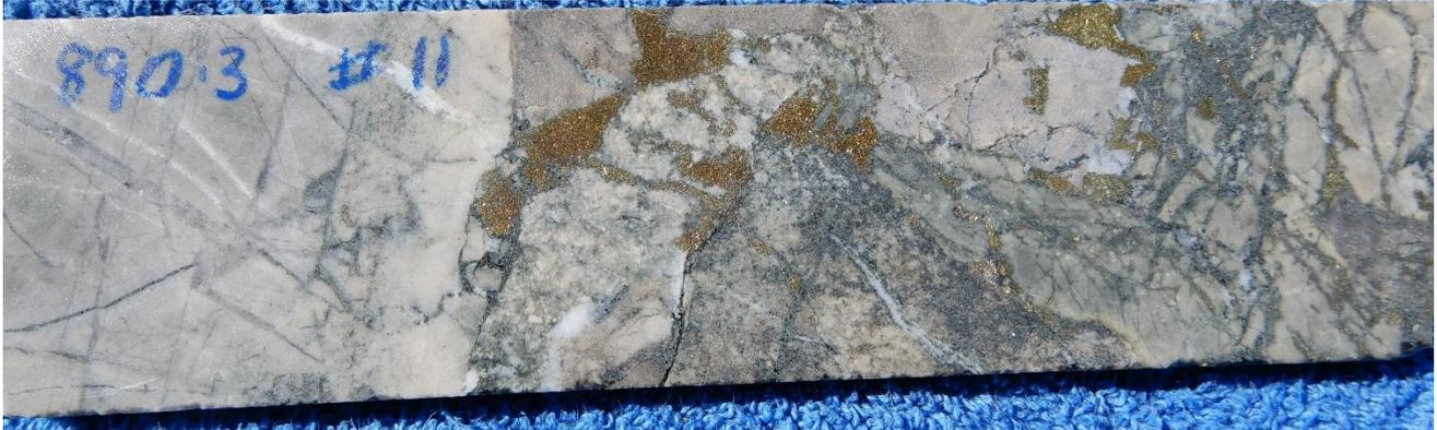
Fig 10. NQ Core photos hole 22CAEDD0011, 890.3m ,Sericitic altered ,clast supported breccia with chlorite -rock flour matrix , pyrite -chalcopyrite chlorite infill. Interval 890m-891m assays 1m @ **10.0 g/t Au 0.46% Cu , , 17.5 g/t Ag, 2.21 % S**
