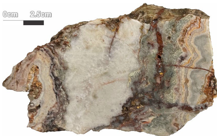
Figure 6. Sample 3927: 4.43g/t Au, 17.4g/t Ag, 90.7ppm Sb colloform-crustiform chalcedony-quartz-carbonate-adularia vein
