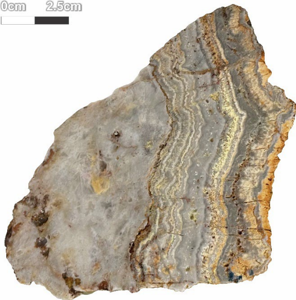
Figure 3. Sample 3946: 1.77g/t Au, 147g/t Ag, 1,810ppm Sb bladed quartz pseudomorphs after calcite with colloform-crustiform banded chalcedony-quartz-adularia veining.
