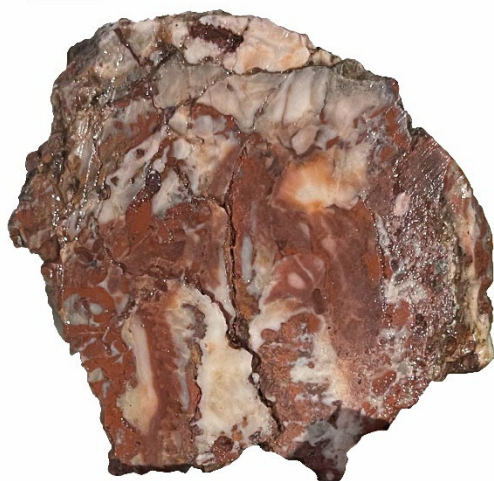
Figure 5. Sample 2951: 17.75g/t Au, 8.3g/t Ag, 28.1ppm Sb, quartz-hematite matrix supported breccia
