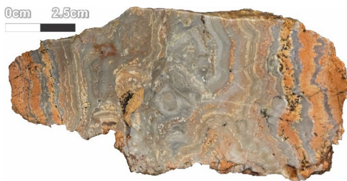
Figure 7. Sample 3933: 1.41g/t Au, 51.4g/t Ag, 1,010ppm Sb Colloform-crustiform chalcedony-quartz-carbonate-adularia vein and locally complex cockade breccia textures.
