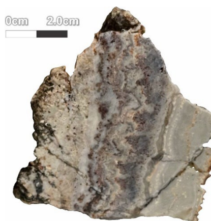
Figure 8. Sample 3926: 1.56g/t Au, 464g/t Ag, 116ppm Sb colloform-crustiform chalcedony-quartz-carbonate vein
