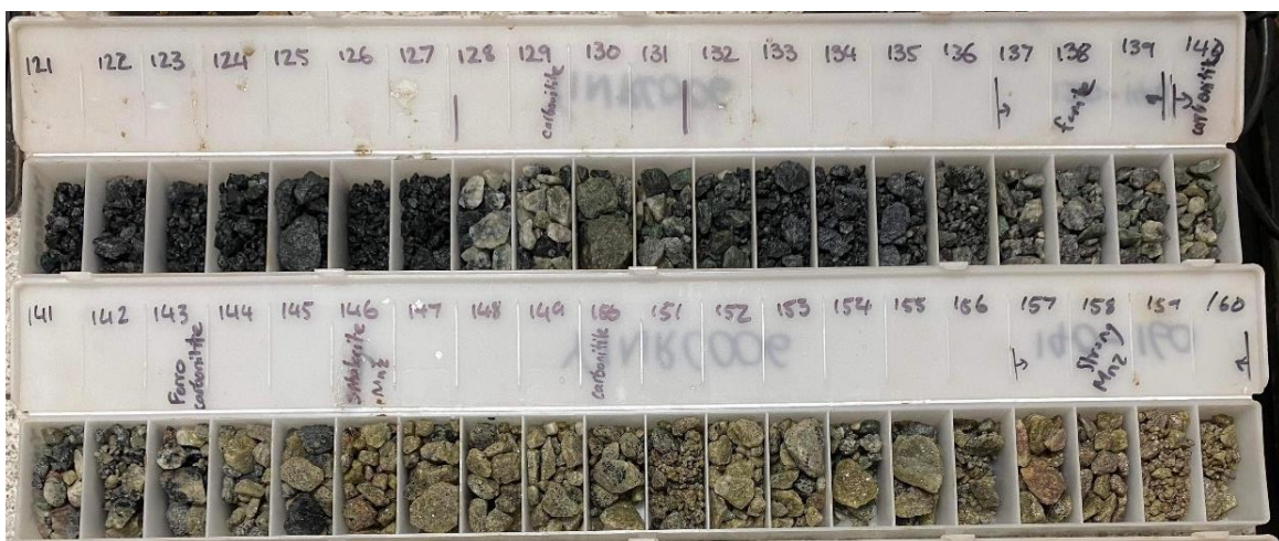
Figure 4: Chip tray from YINRC006 showing dark fenitic alteration grading into two mineralised fresh ironstones (ferrocarnatite) from 127-131m and 139m-160m.
