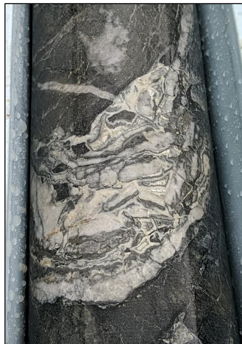
Figure 3: 10cm wide crustiform quartz-adularia-sulphide vein breccia from 146m in PPDH182 Apollo twin hole. (assays pending, vein located proximal to mineralisation in twin hole PPRC826)
