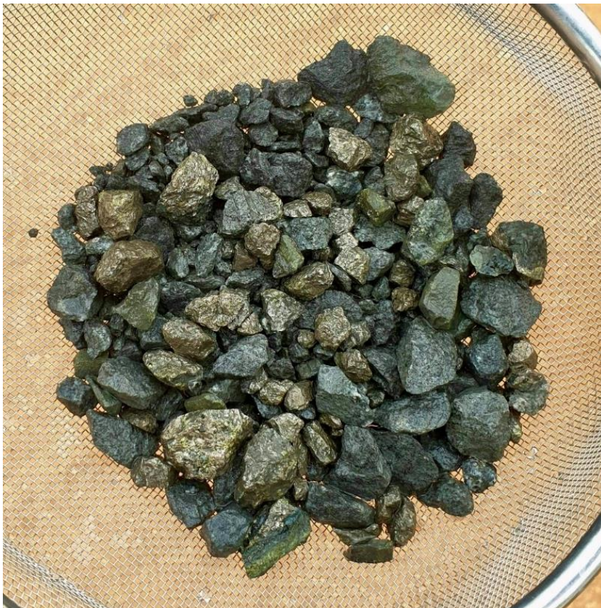
Figure 1: RC chips from REYRC002 79-80m showing net-textured / brecciated Ni-Cu sulphides (~15-20%) comprised of pyrrhotite, chalcopyrite and pentlandite.
