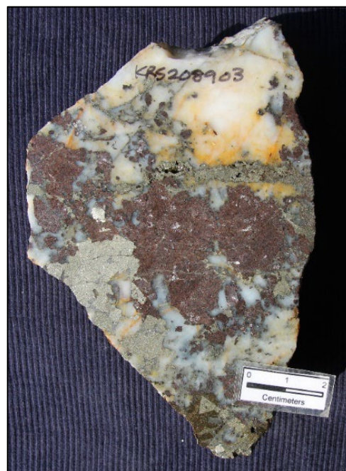
Figure 11: Magnetic pyrrhotite clots, pyrite and sphalerite in re-brecciated comb vein quartz from mullock dump at Darae mine. Sample KRS208903, 41.4 g/t Au 55.3 g/t Ag.
