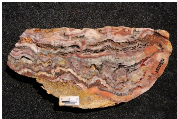
Figure 5: Mineralised Colloform banded vein clast in conglomerate, pre-dating mineralisation at Geoje mine. Sample KRS505511, 0.26 g/t Au 0.20 g/t Ag.
