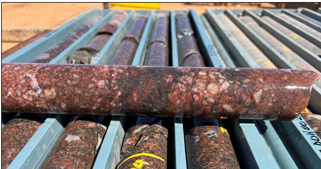
Figure 1. Felsic intrusive breccia containing significant hematite alteration with hematite and minor magnetite and pyrite within the matrix (HELIOS_DD002)
