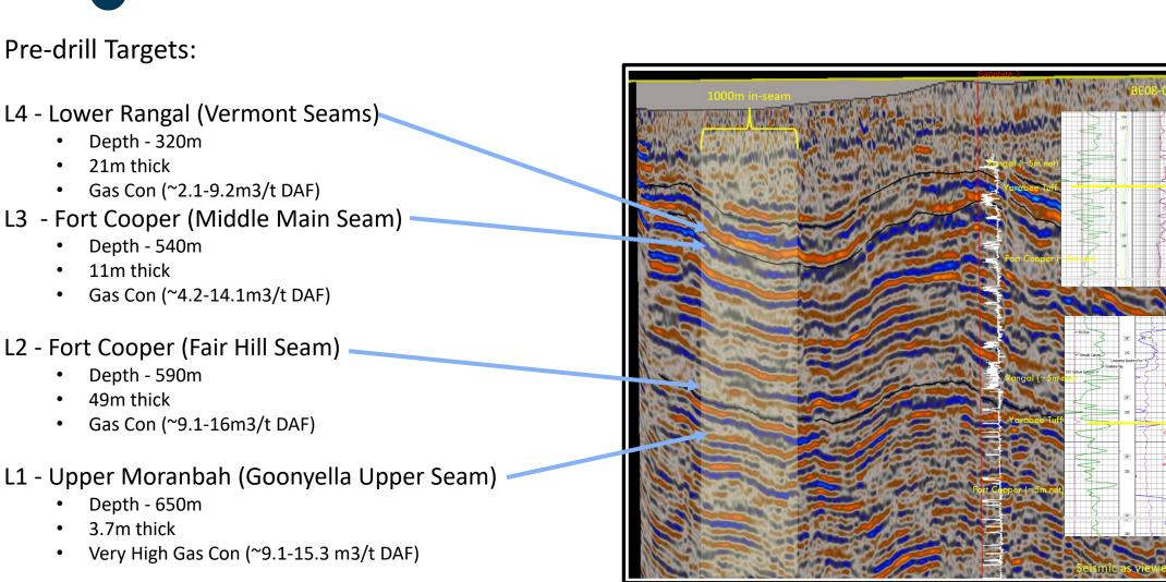
Deepest target seam targeted by L1 Lateral – drilled first for control of shallower targets
