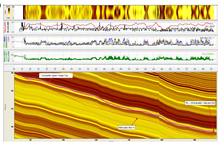
Successfully geo steering in the coal. Use of near bit gamma has enabled almost 100% in coal for the first lateral
