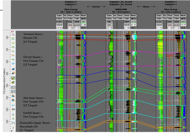
Fair Hill Seam (L2) target changed to the Girrah seam (Fort Coopers - Leo seam) after vertical well data obtained Targets now:
