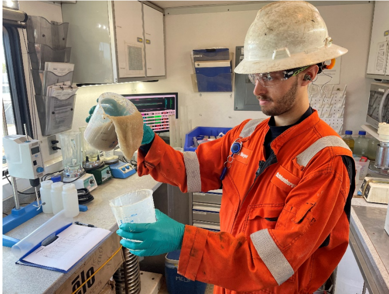
Testing crosslink hydraulic stimulation fluid during Carpentaria-2H operations
