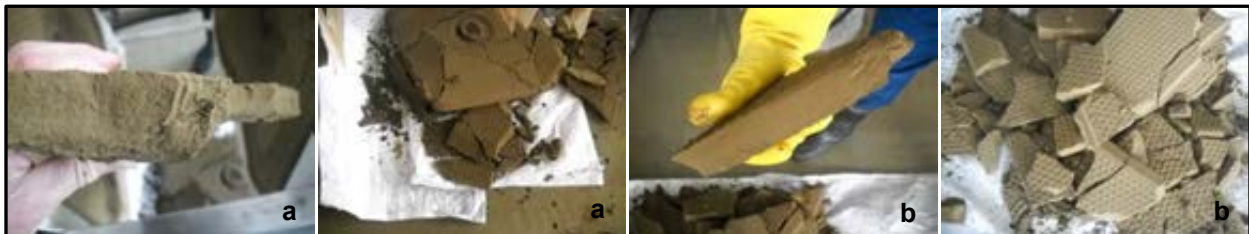
Figure 13-30: Filtration Cakes – Leach Residue (a: 26.4% w/w Moisture; b: 24.7% w/w Moisture)
