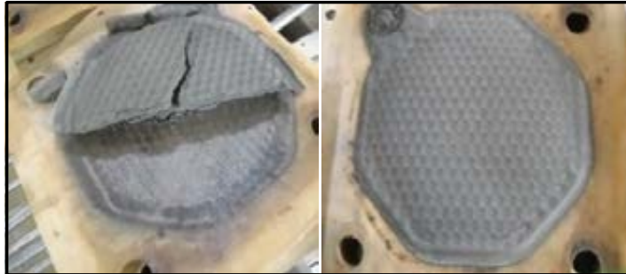
Figure 13-29: Filtration Cakes – Non-Magnetic Tailings (12.6% w/w Moisture)
