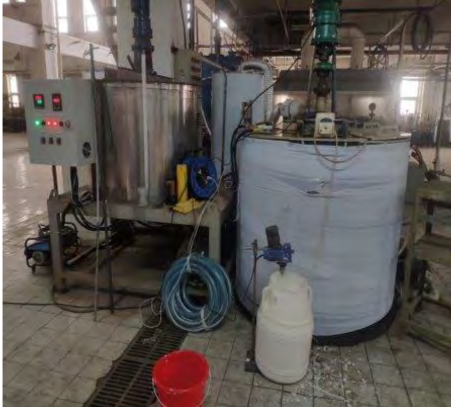
Figure 13-23: Leaching Testing for Preparing Slurry for Dewatering Tests
