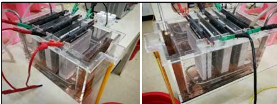
Figure 13-25: One of Electrowinning Test Devices
