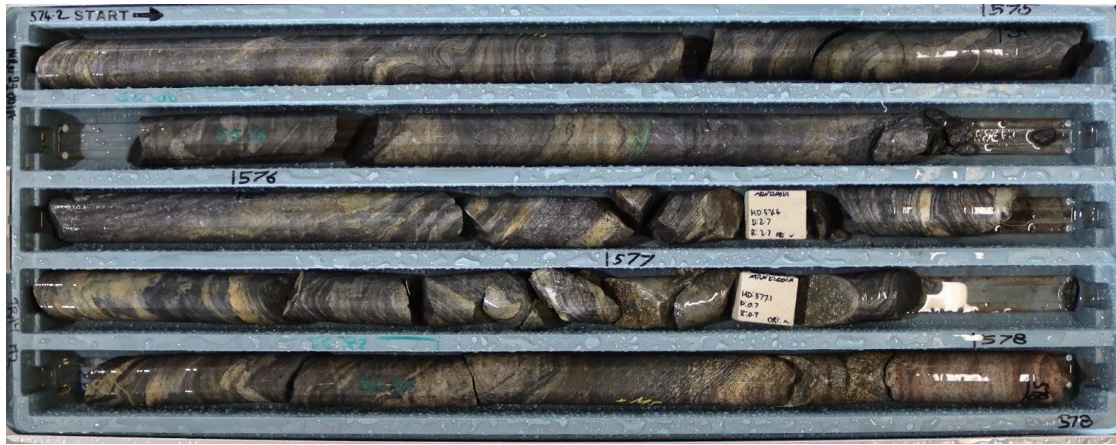
Figure 2. Example of mineralised Western Pb-Ag horizon in MRN22001A (574.2 - 578m downhole)
