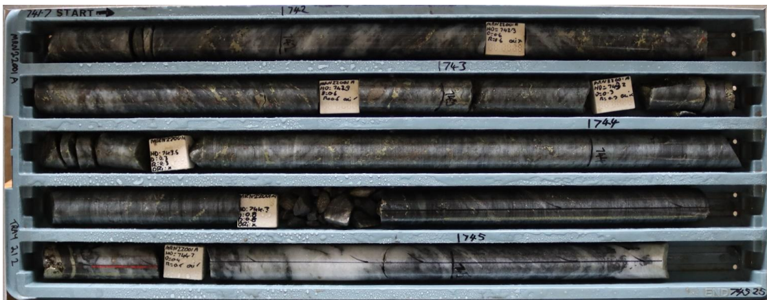
Figure 4. Example of higher tenor Pyrrhotite-Pyrite-Chalcopyrite mineralisation in MRN22001A (741.7 - 745.25m downhole)
