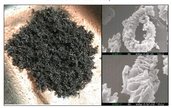
Figure 9: 220% Expansion Factor for +60 Mesh (+250 micron) sized flake.
