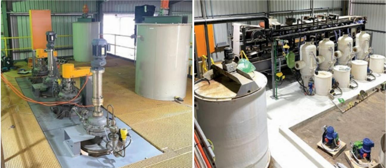
Figure 4 – **Demonstration Plant. Left: Iron oxidation and precipitation circuit. Right: Installation of iron polishing and MHP precipitation circuits.**
