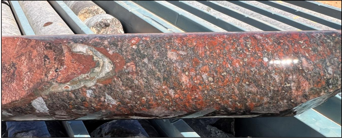
Figure 9. Photo of drill core (HELIOS_DD002) at approximately 1000m depth. The image photo shows the broken nature of the granite with hematite alteration. NQ drill core Ø ~47mm.
