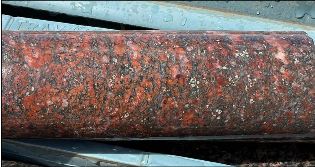
Figure 3. Pervasive iron oxide staining (red) together with hematite (grey) minor magnetite and sericite alteration of the host granite (HELIOS_DD002). NQ drill core \varnothing ~47mm.
