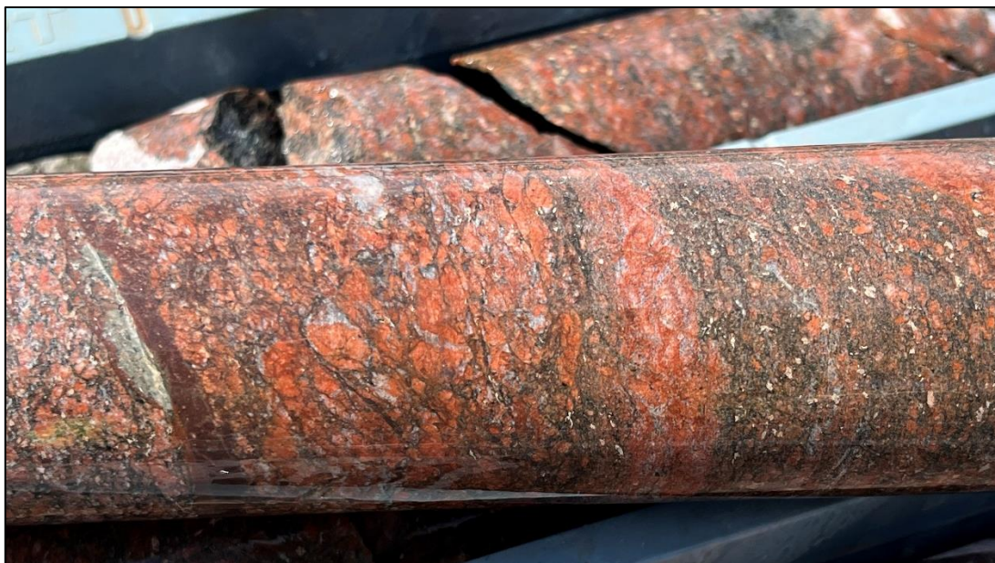
Figure 7. Photo of drill core (HELIOS_DD002) at approximately 990m depth. The image photo shows the broken nature of the granite with hematite alteration. NQ drill core \varnothing ~47mm.
