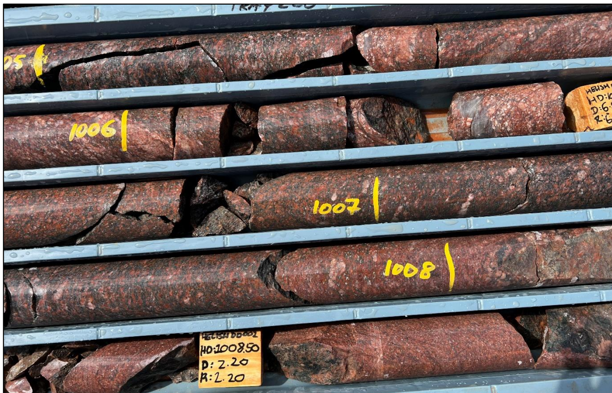
Figure 1. Felsic intrusive breccia containing significant hematite alteration with hematite and minor magnetite and pyrite within the matrix (HELIOS_DD002). NQ size drill core. Yellow numbering represents down-hole depth in meters.
