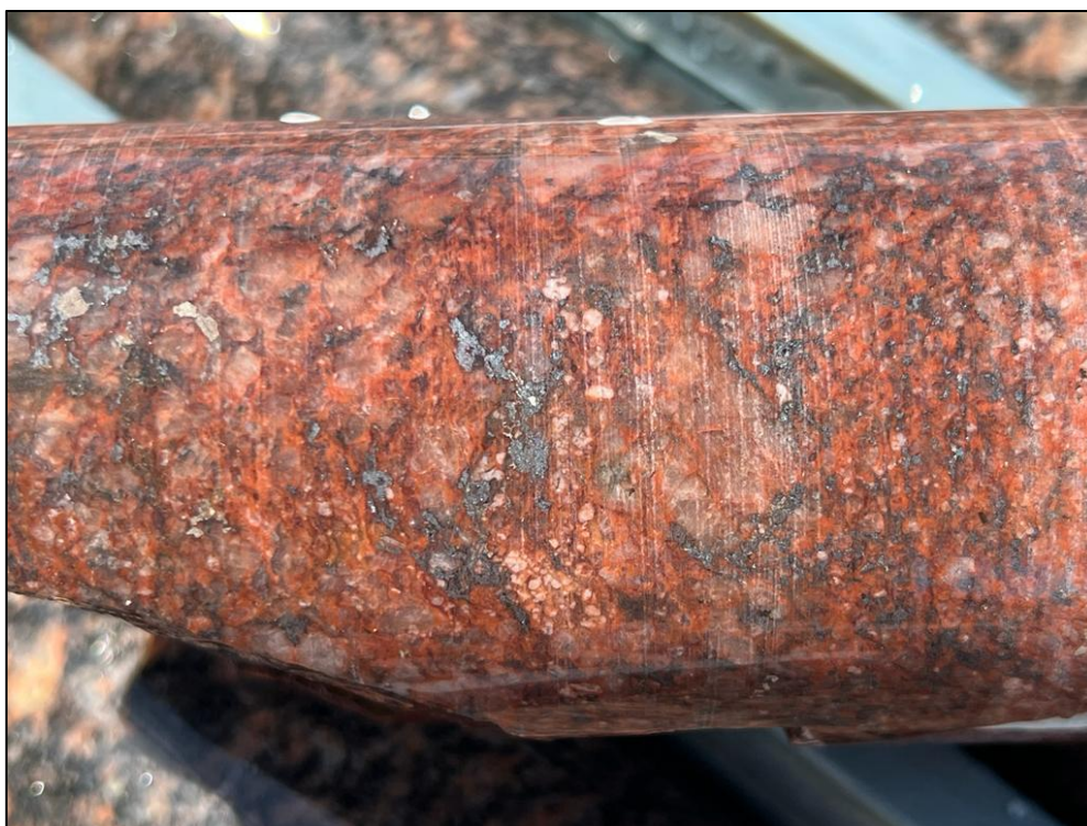
Figure 2. Pervasive iron oxide staining (red) and intergranular hematite (silver grey) in altered granitic host rocks (HELIOS_DD002). NQ drill core \varnothing ~47mm.
