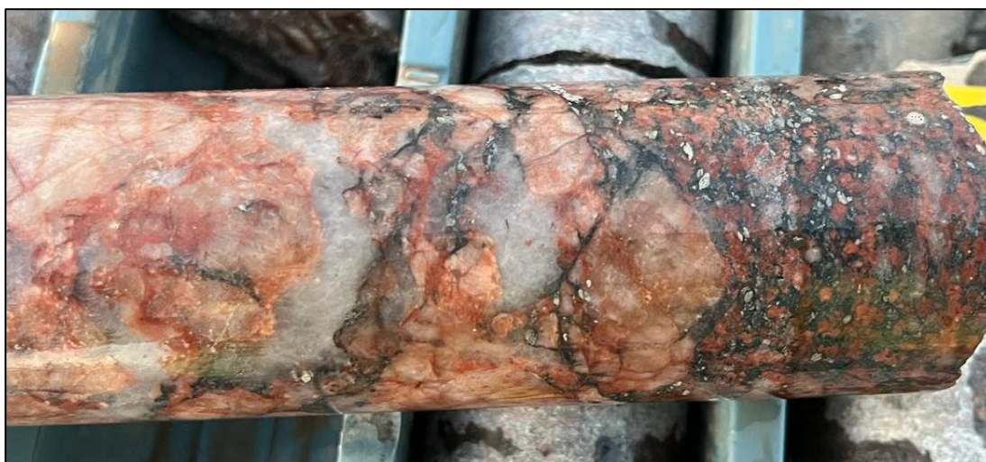
Figure 8. Section of drill core from HELIOS_DD002 (NQ diameter) showing the contact between a pegmatitic (coarse-grained) part of the host granite and the altered, sericite, hematite, and hematite altered granite. NQ drill core \varnothing ~47mm.
