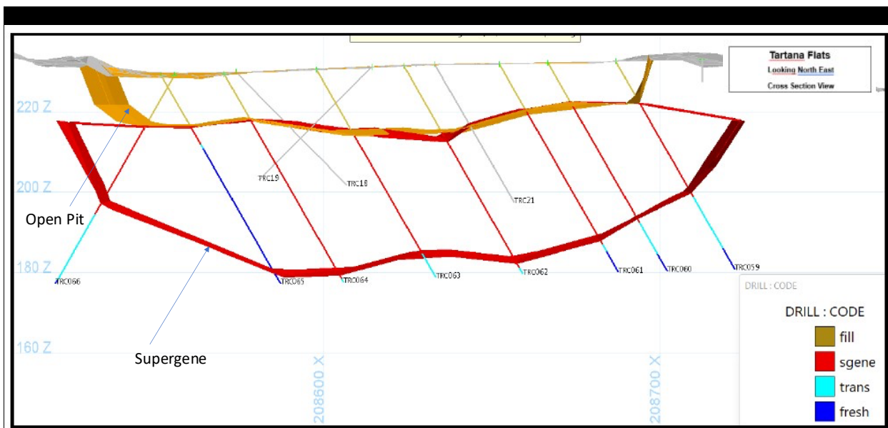
Figure 3. Cross-section of the most southerly fence-line in the north portion of the pit. Supergene zone in red with transition and primary ore below. The overlying fill is above the ore zone. Source: BMS.
