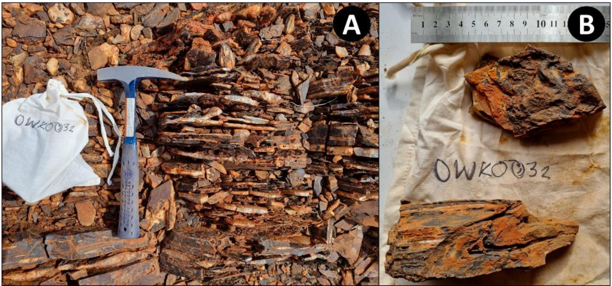
Figure 7A – Laminated ferruginised chert/shale beds sampled for sample OWK0032. 7B – Hand specimen collected for assay
