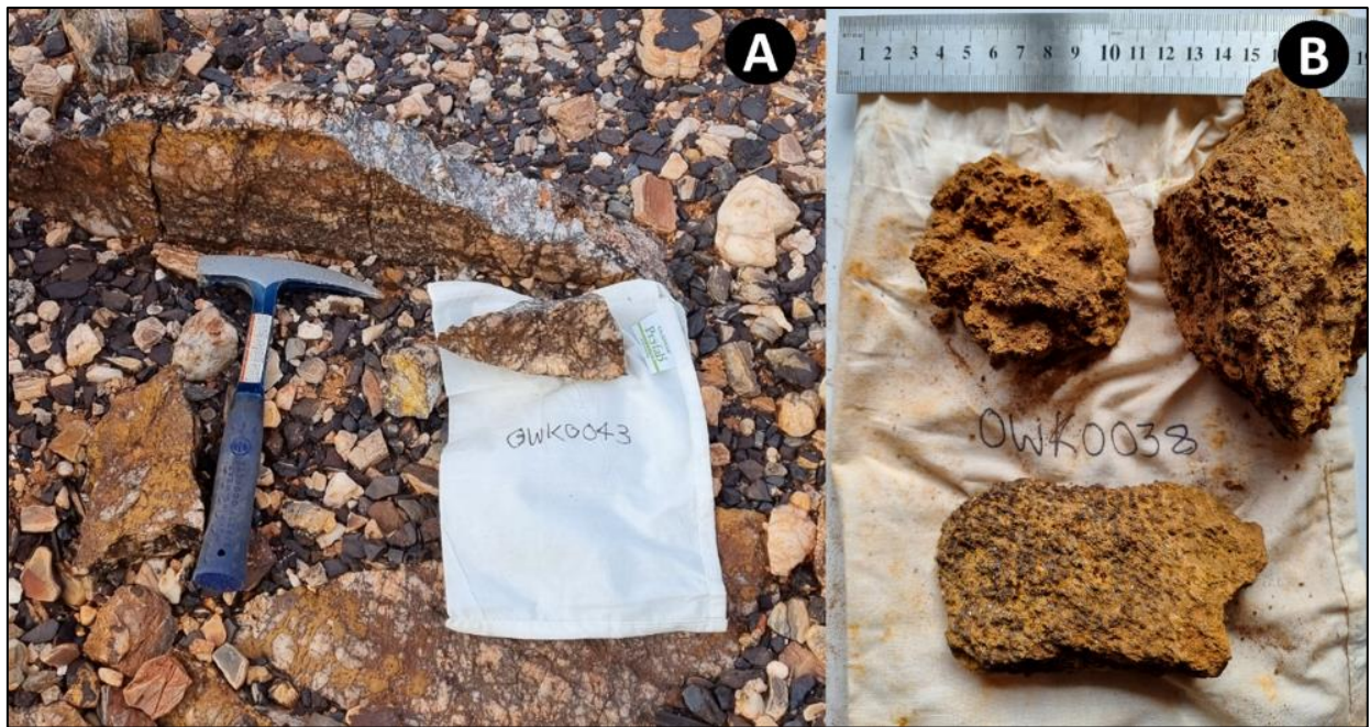
Figure 8A – Brecciated Geothitic Quartz vein. 8B – Weathered ultramafic with relict texture
