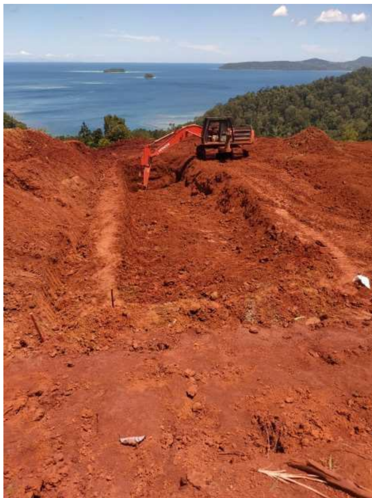
Photo: Saprolite ore being dug for stockpile
