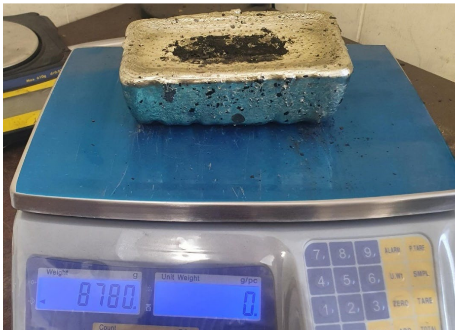
Gold Doré Bar containing Gold and Silver bullion poured from gold stripped from carbon 28/09/2022
