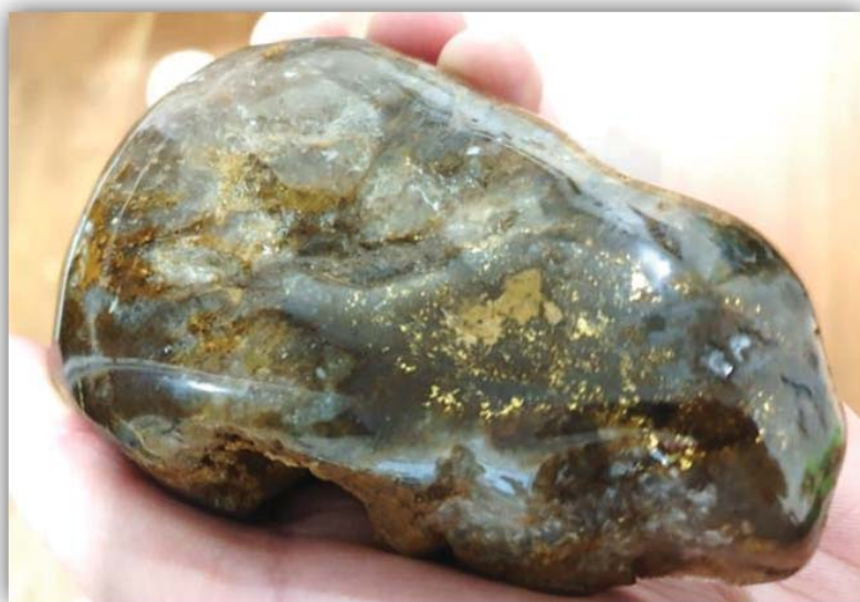
Figure 2: Photograph of polished gossanous quartz vein with abundant visible gold recently sampled by the Company from the outcrop exposures in the north face of the Brians historic pit.
