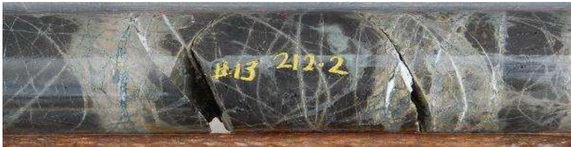
Fig 18 HQ Full Core photos hole 22CAEDD0013, 212.2m, Structural preparation evident with multi-directional & multi-generational quartz pyrite vein stockwork with alteration selvages cutting & bleaching biotite hornfels.
