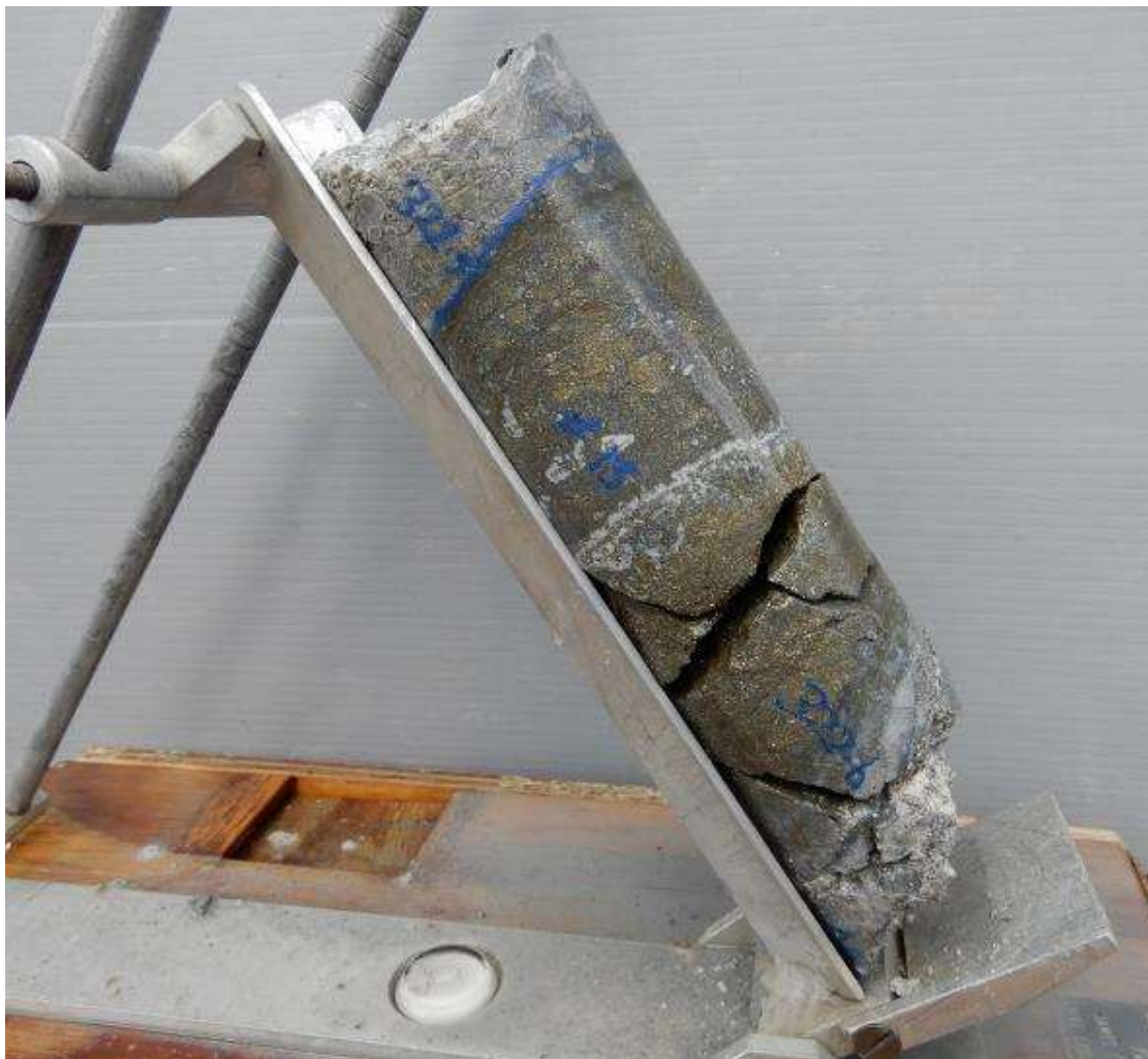
Fig 21. HQ Full Core oriented in Core Orienting Frame, hole drilling south-west (hole bearing 219 degrees mag) inclined at 61 degrees, view looking south-east. Hole 22CAEDD013 at 322.6m: brecciated high-grade gold bearing massive sulphide infill within strongly sericite-silica altered and veined fault zone. Measured dip of sulphide vein - 45 degrees towards 030 (north north-east). Interval 322m-323m 1m grading 0.22% Cu, 22.98 g/t Au, 60 g/t Ag, 7.62% S, 0.54% Pb, 94 ppm Bi.
