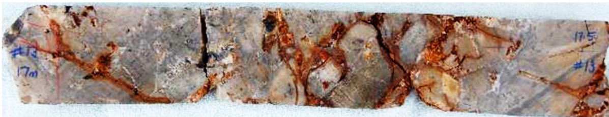
Fig 11. HQ Half Core photos hole 22CAEDD0013, Near surface gold bearing, partially oxide material . Gossanous hydrothermal infill breccia dominated by hornfels clasts, infill quartz ,oxidised sulphide @ 17m depth. Interval 17m-17.5m : 0.5m grading, 22.7 g/t Au, 10.7 g/t Ag, 0.52% Cu, 1.88% S.
