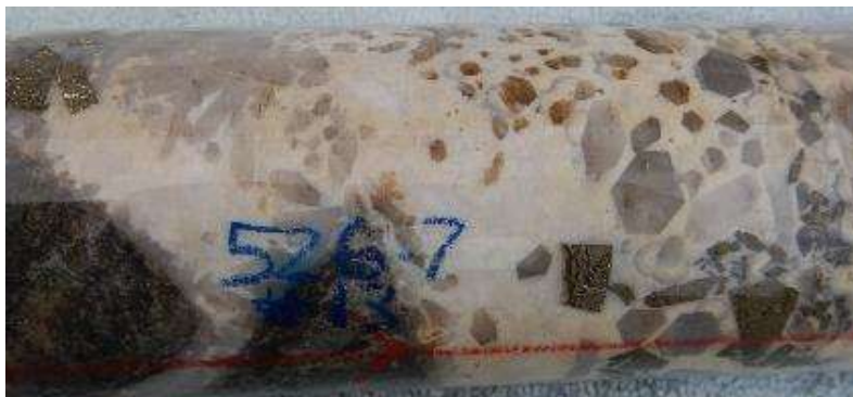
Fig 22 HQ Full Core photos hole 22CAEDD0013, 496.05m ,514.9m. Quartz - Molybdenite as veins & fracture coatings within clasts of carbonate (+/- K feldspar? altered diorite & porphyry in clast supported breccia. Prominent matrix infill of quartz, and coarse calcite. Evidence of a higher temperature core of intrusive mineral system (porphyry style?) as hole drills to south-west. Intervals 496m-497m 1m grading 138 ppm Mo. 514m-515m 1m grading 117 ppm Mo.
