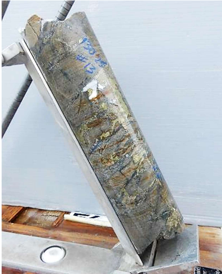
Fig 15. HQ Full Core oriented in Core Orienting Frame, hole drilling south-west (hole bearing 218 degrees mag) inclined at 63 degrees, view looking south-east. Hole 22CAEDD013 at 130.25m: slab like hornfels clasts generally aligned in layers, dipping east. chalcopyrite -pyrite-calcite-quartz infill. Interval 130m-131m grading 2.24% Cu, 0.56 g/t Au,30 g/t Ag, 9.2% S.
