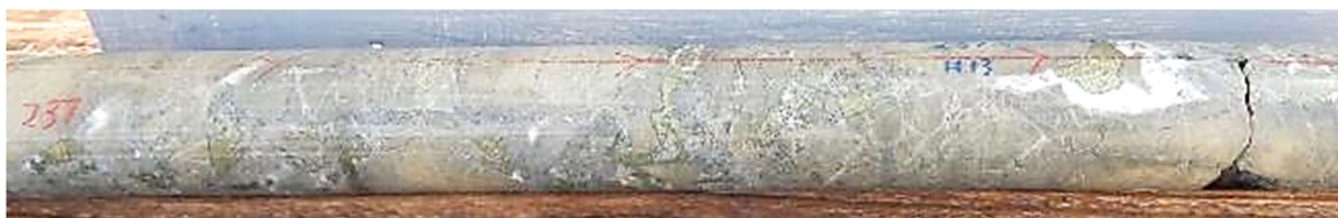
Fig 16. HQ Full Core photos hole 22CAEDD0013, 233.5m,237.4m , Chalcopyrite – pyrite-quartz – calcite infill between angular clasts of sericite altered hornfels. Interval (top) 233m-234m grading 1.77% Cu, 0.43 g/t Au,25 g/t Ag,7.95% S; (bottom) 237m-238m grading 1.88% Cu, 0.23 g/t Au,21.8 g/t Ag,.5.49% S.
