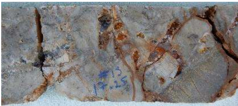
Near surface, gold bearing gossanous hydrothermal infill breccia CAE hole # 13: 17m depth. Interval 17m-17.5m: 0.5m grading, 22.7 g/t Au, 10.7 g/t Ag, 0.52% Cu.
