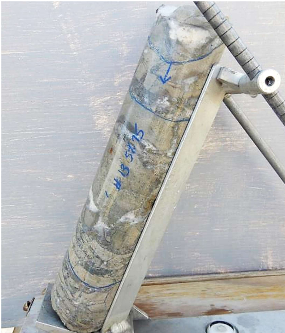
Fig 14. HQ Full Core oriented in Core Orienting Frame, hole drilling south-west (hole bearing 214 degrees mag) inclined at 64 degrees, view looking north west. Hole 22CAEDD013 at 57.75m : slab like hornfels clasts generally aligned in layers, measured dip of layering of clasts is -40 degrees towards 070 (east north east).
