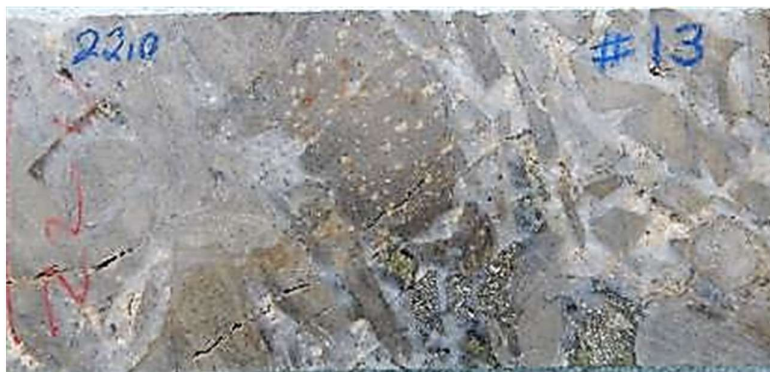
Fig 11. HQ Half Core photos hole 22CAEDD0013, Near surface gold bearing, partially oxide material . Gossanous hydrothermal infill breccia dominated by hornfels clasts, infill quartz ,oxidised sulphide @ 17m depth. Interval 17m-17.5m : 0.5m grading, 22.7 g/t Au, 10.7 g/t Ag, 0.52% Cu, 1.88% S.
