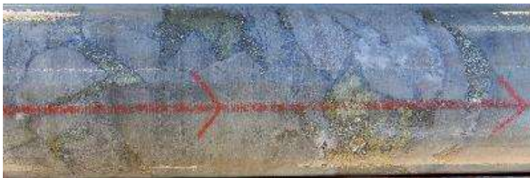
Typical clast supported breccia dominated by sericite altered hornfels clasts, chalcopyrite -pyrite -calcite-quartz infill. CAE hole # 13, : 52m depth.
