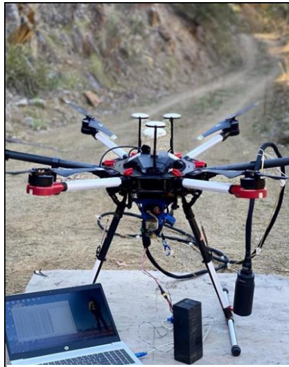
Image 1 - UAV's utilised to complete the drone magnetic survey at Gunnawarra.
