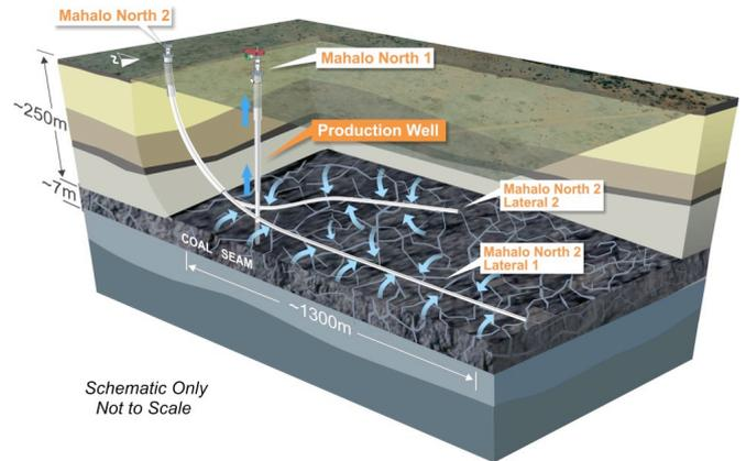
**Figure 5 – Cutaway diagram of the Mahalo North 1 and Mahalo North 2 pilot well**
