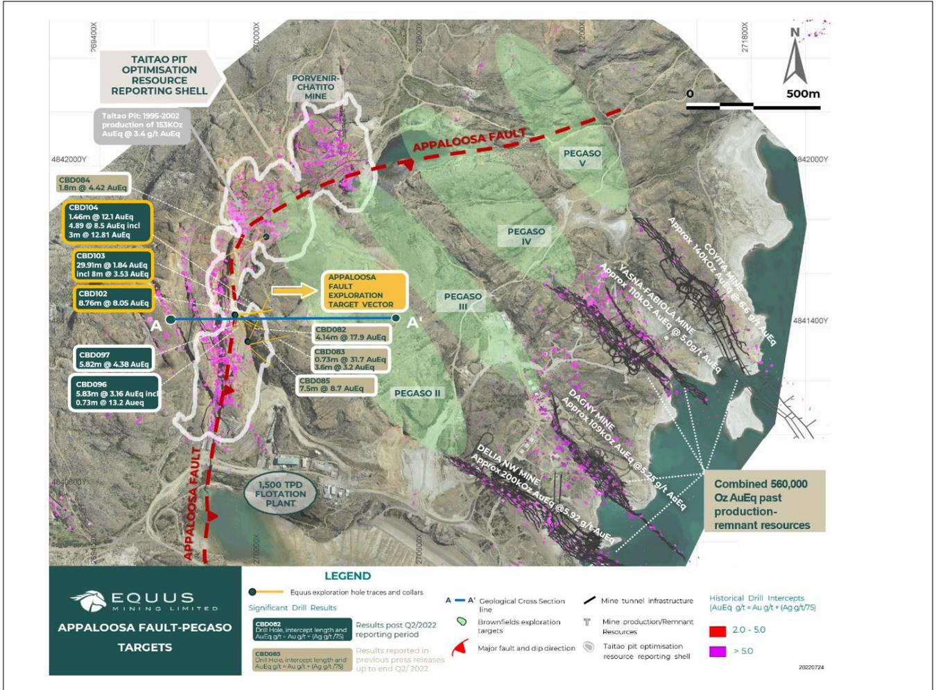
Figure 4 – Plan view showing location of the Taitao-Appaloosa Fault, Pegaso II- V targets, location of cross section A -A' (see Figure 5) and historic underground mine workings and summary resources of the Delia, Dagny, Fabiola and Coyita Mines, and historic production of the Taitao Pit.
