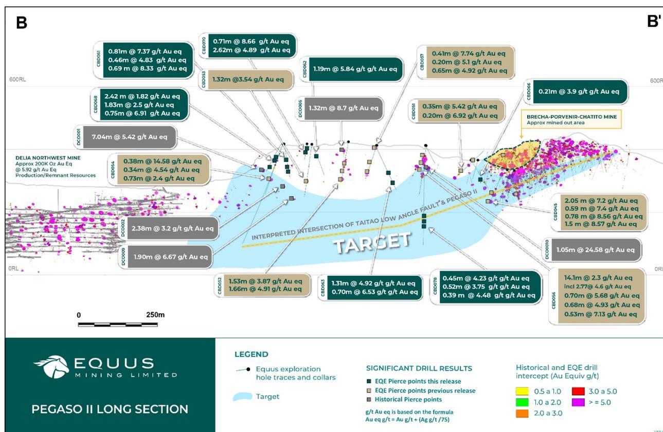
Figure 7 - Pegaso II long section B-B' - showing summary Equus and historic drill result pierce points, interpreted exploration target at the intersection of the low angle Appaloosa Fault and subvertical Pegaso II structure and underground mine workings of the Delia NW mine
