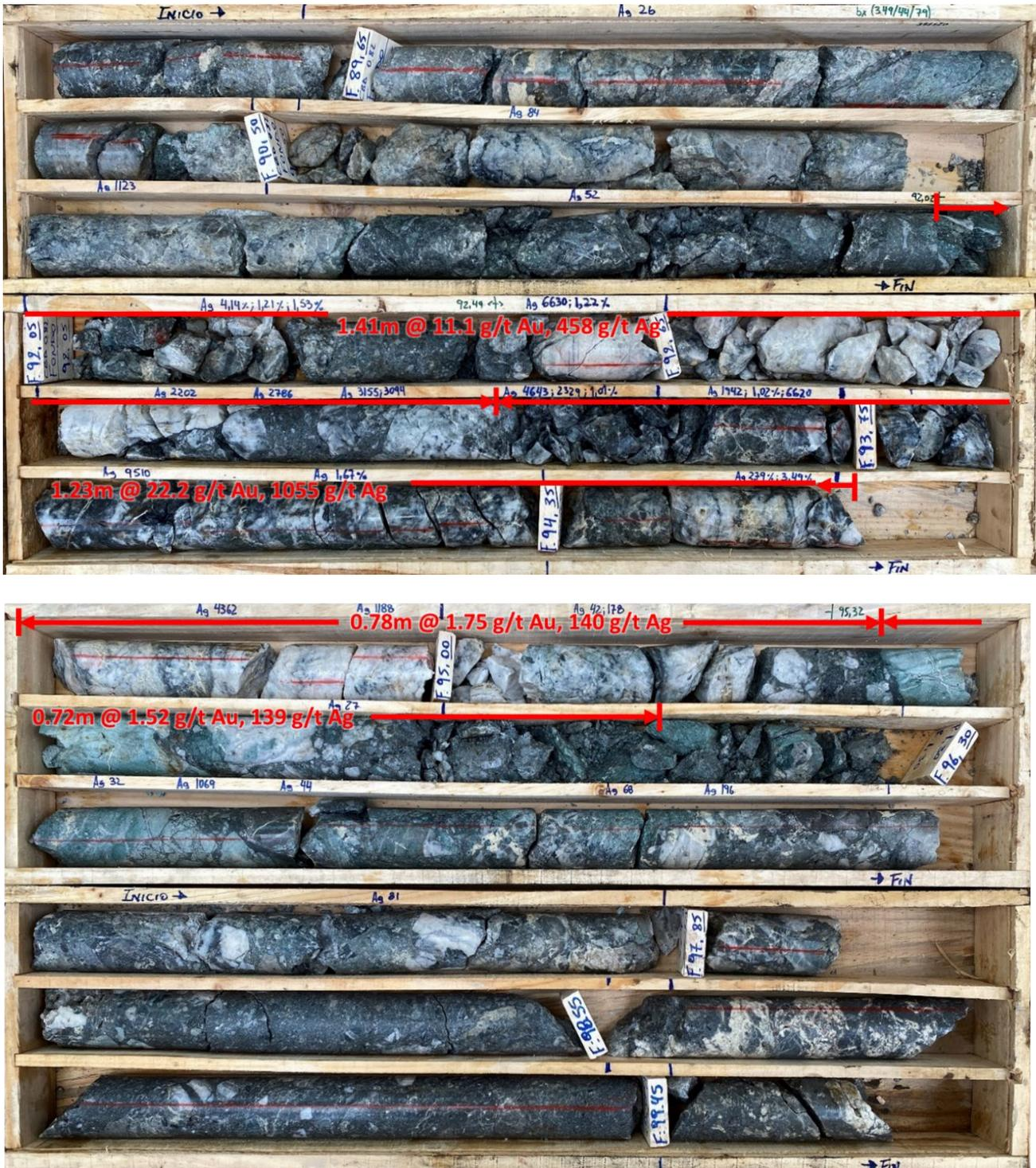
Photo 1. CBD102 drill core displaying the high grade epithermal vein-breccia interval which returned 4.14m @ 17.9 g/t AuEq<sup>2</sup> (11.0 g/t Au, 520.0 g/t Ag) from 92.01m -96.15m including 2.64m @ 26.1 g/t AuEq<sup>2</sup> (16.3 g/t Au, 736.1 g/t Ag) from 92.01-94.65m
