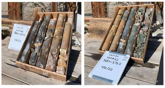
Figure 8: Altered and mineralised target zone intersected in DCD-01
