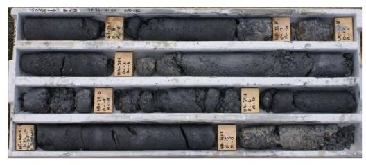
Figure 3: Original core from OAD002, (containing 1.7m @ 16.65% TGC from 39.60m), prior to sampling and resampling for the new testwork to feed into the updated scoping study
