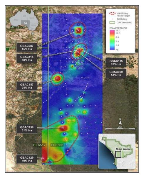
Figure 5: Gibraltar Project with all aircore drill collars and maximum down-hole halloysite value contours plus selected composite results
