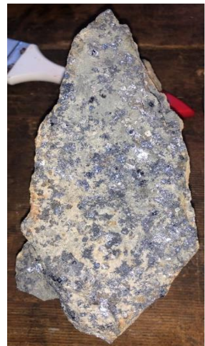
Webbs Consol Main Shaft specimen showing coarse galena mineralisation
