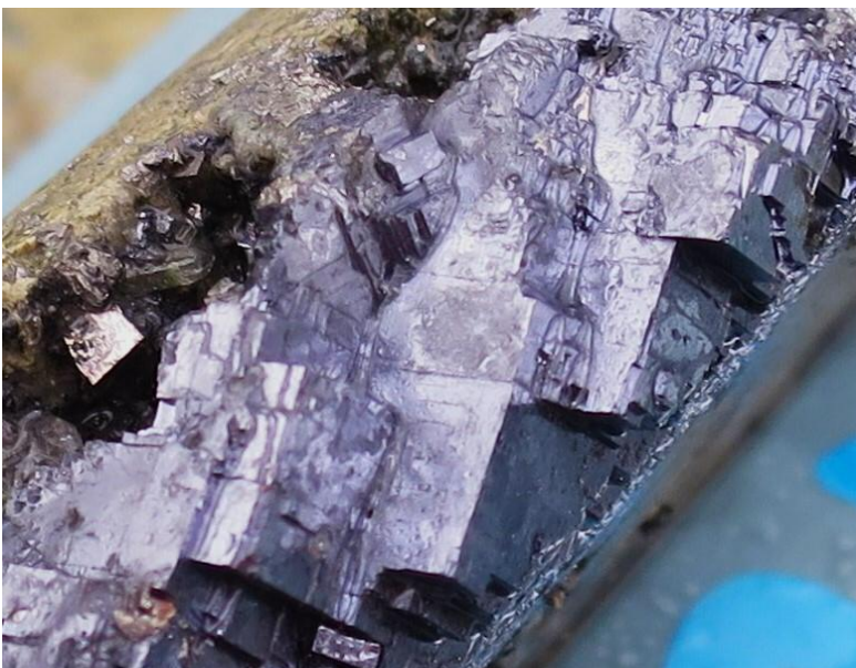
Photo 1: Massive galena (PbS) vein in core at 112.4m depth in drill hole WCS031 (NQ2 half core). Galena presented as very coarse euhedral crystals with classic cubic crystal habit.
