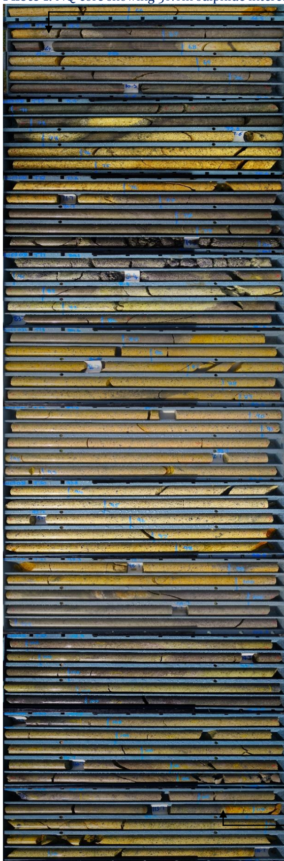
Photo 1: NQ core showing 50.0m sulphide intercept from drill hole WCS031 at Castlereagh prospect
