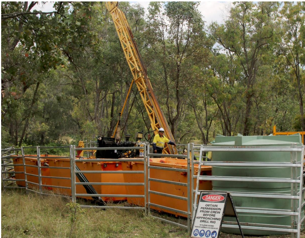
Figure 1 Core drill rig during initial set-up at the Northern Porphyry target at Briggs
