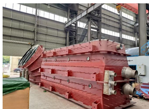
Figure 4: Andritz, Draft Tube Liner - September 2022
