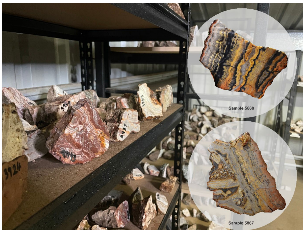
Figure 1: The Bauloora Epithermal Gold Project Rock Library showing an extensive catalogue of surface rock samples obtained and logged during the systematic mapping of the vein field 1 . Surface rock samples 5867 and 5868 show well developed quartz (white-very dark grey)-chalcedony (grey/white)-adularia (yellow-orange) colloform-crustiform banding and breccia with 0 - 5 trace % sulphides estimated 1 , and assays pending.
