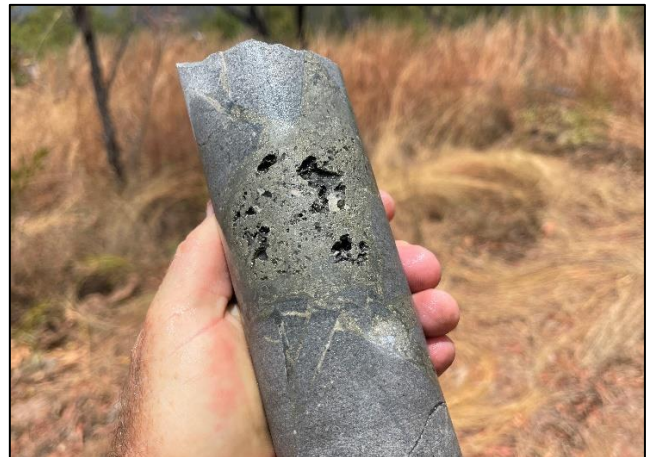
Figure 1. First sections of core recovered during the first 134m of drilling MPD002 at Maneater Hill. The drill core between approximately 107m and 116m down-hole depth contains abundant sulfides and confirms the presence of sulfide-rich, polymetallic breccias at the Maneater prospect. All core is HQ3 diameter.
