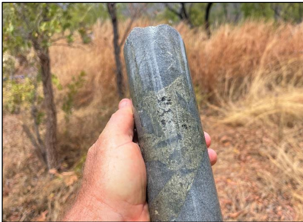
Figure 1. First sections of core recovered during the first 134m of drilling MPD002 at Maneater Hill. The drill core between approximately 107m and 116m down-hole depth contains abundant sulfides and confirms the presence of sulfide-rich, polymetallic breccias at the Maneater prospect. All core is HQ3 diameter.
