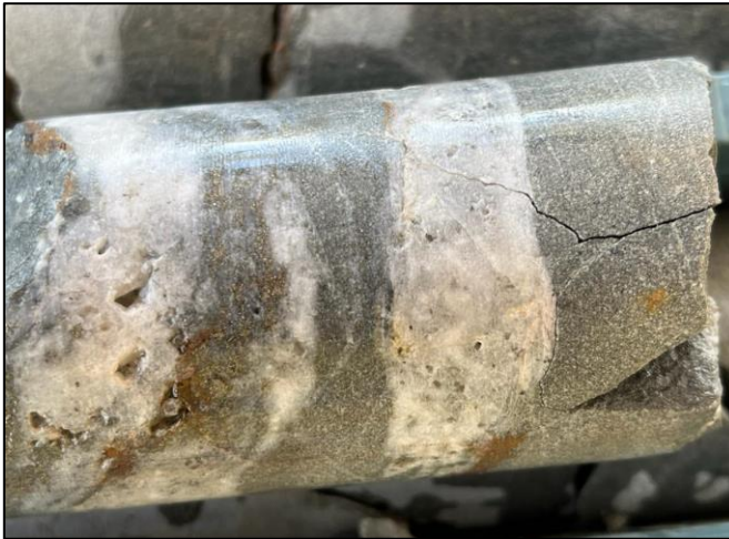
Figure 4. Quartz-Carbonate veining cutting altered Hodgkinson Province metasandstone. MPD002 HQ3 diameter.
