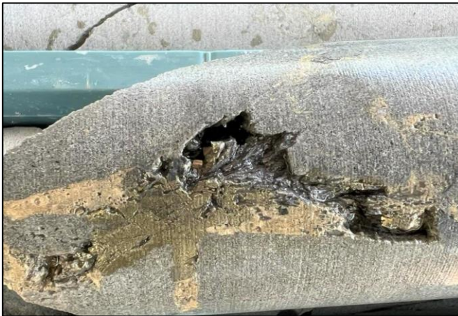
Figure 5. Sulfide-Carbonate in altered metasandstone host rock. Sulfide assemblage includes pyrite, sphalerite, and galena (to be confirmed). MPD002 HQ3 diameter.
