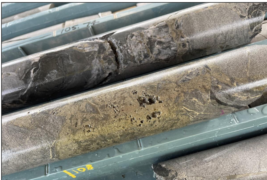
Figure 2. Photo of massive sulfides (predominantly pyrite in this section of core) infilling altered meta-sandstone breccia. (MPD002 108.6m depth down hole). HQ3 diameter drill core.
