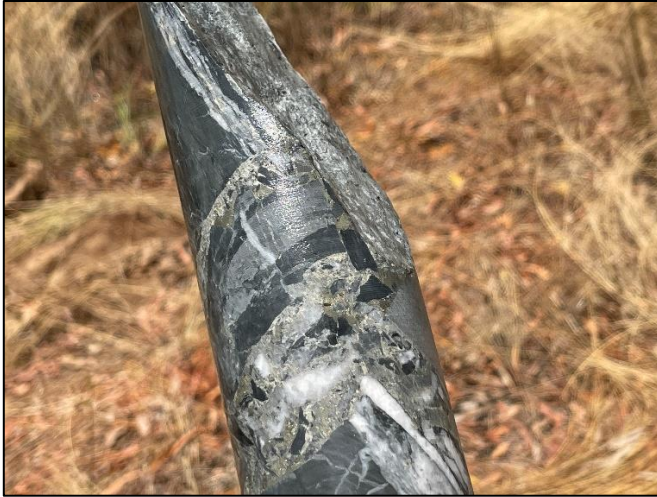
Figure 3. Photo of brecciated metasediments with quartz, carbonate, sulfide infill. (MPD002 107.4m depth down hole). HQ3 diameter drill core.
