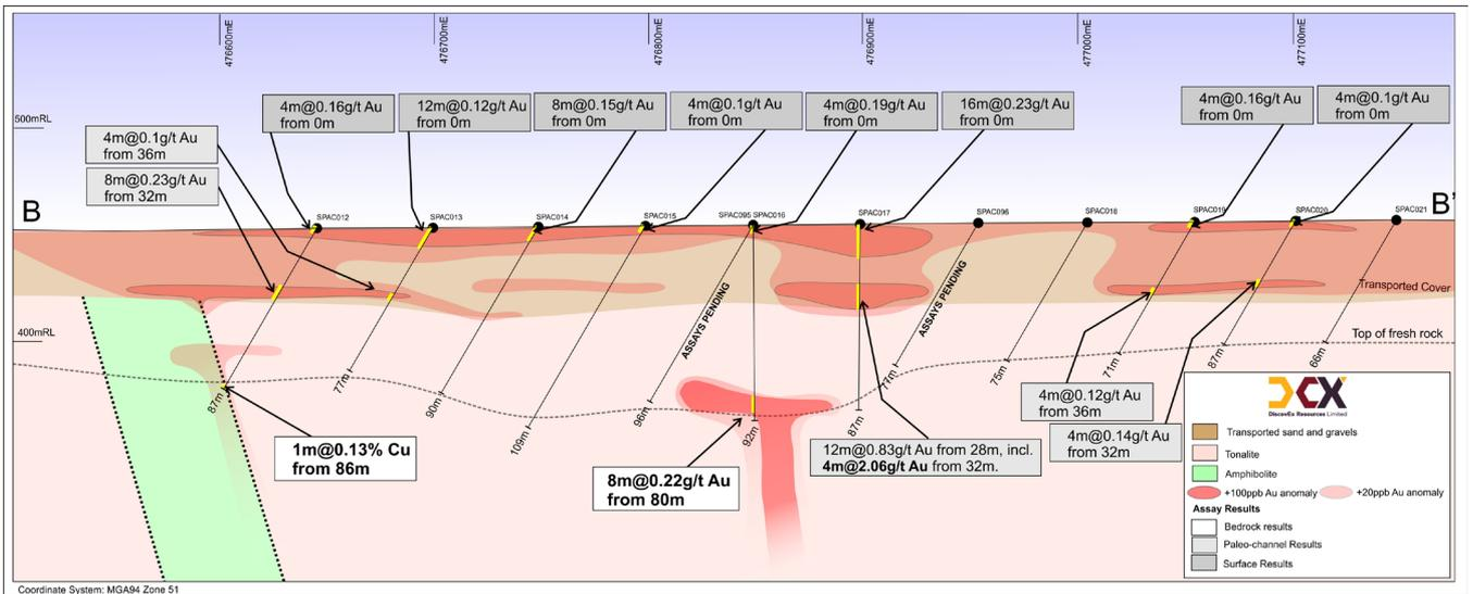
**Figure 3: Drillhole section 6716950mN**
