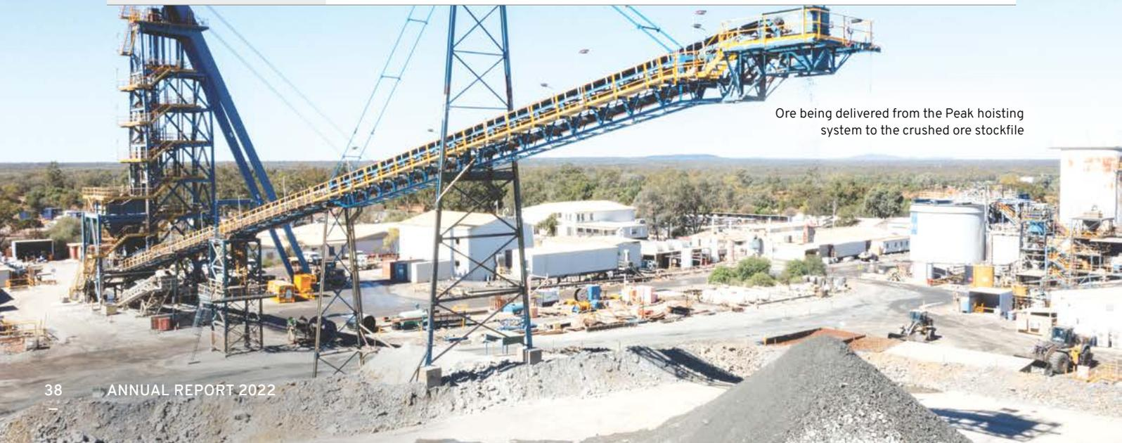
Ore being delivered from the Peak hoisting system to the crushed ore stockpile
