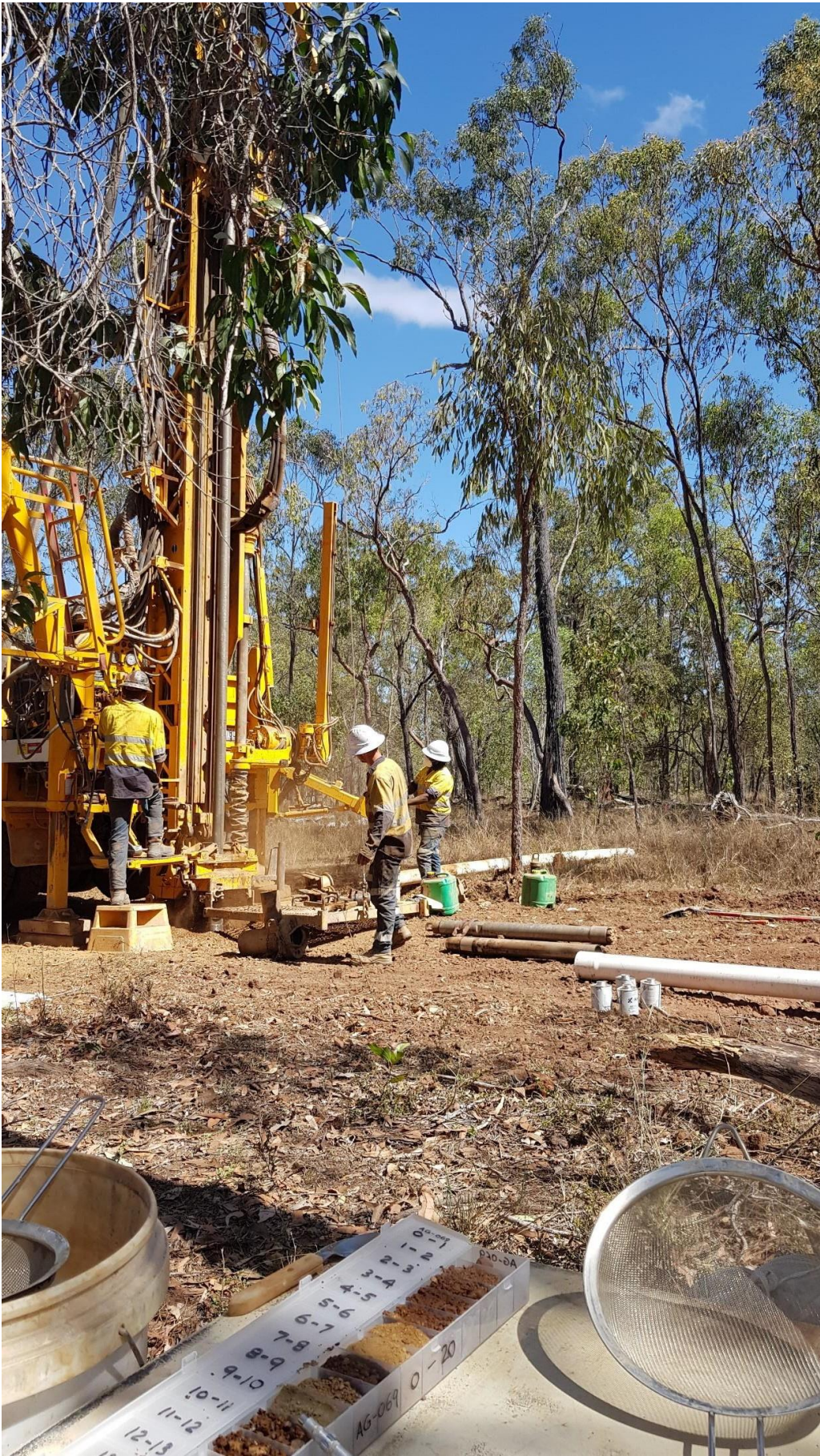
Figure 1: RC drilling the Pod at Gunnawarra North Queensland
