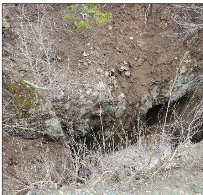
Figure 1 - Adit providing access into the historical workings
