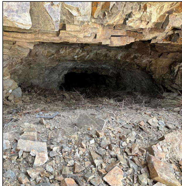
Figure 8 – Historical Adit following a highly altered near parallel quartz vein. The highly altered white quartz vein was directly adjacent to the shear zone
