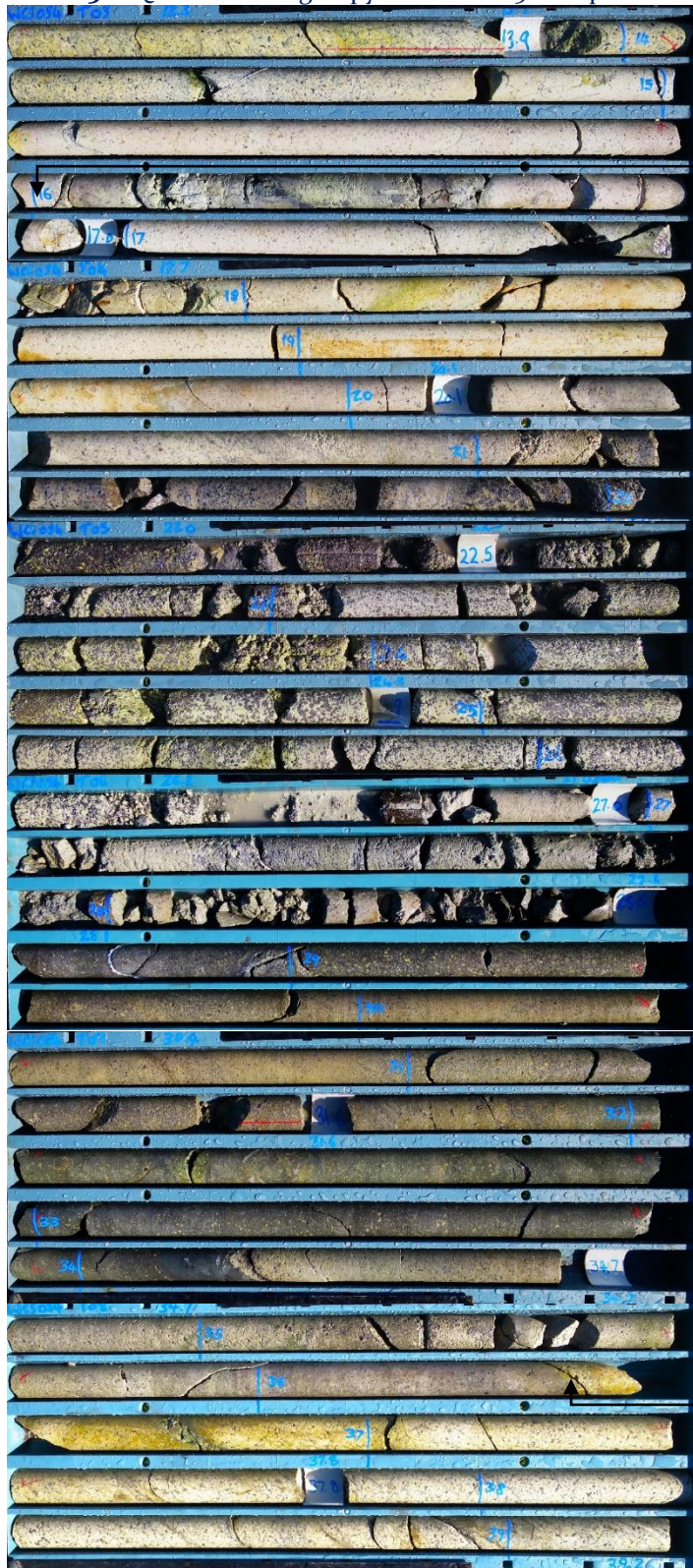
Photo 3: NQ core showing Copycat Lode 20.5m sulphide intercept from drill hole WCS034
