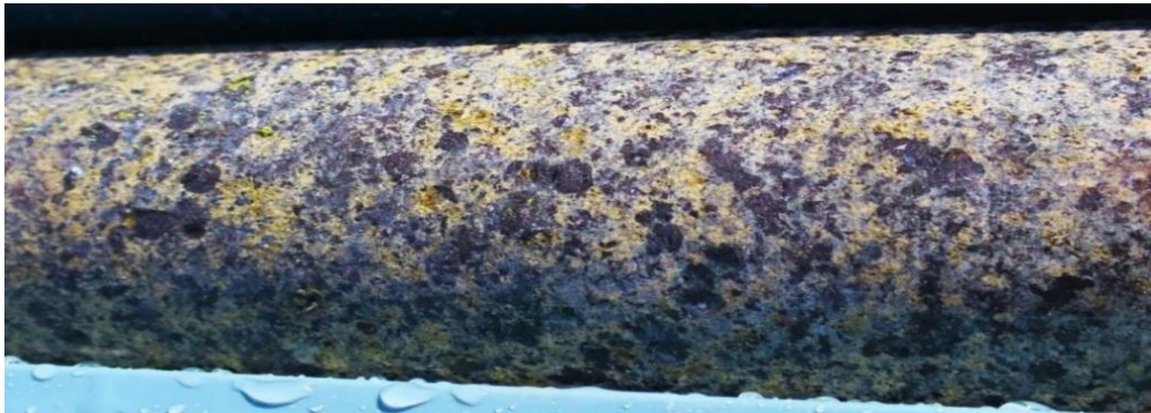
Photo 2: Coarse sphalerite ((Zn,Fe)S) mineralisation at 21.5-21.7m depth in hole WCS034 (NQ2 core)
