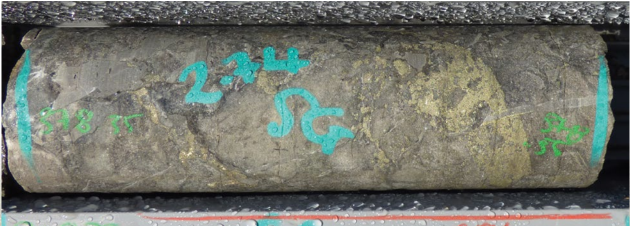
Figure 4: Drill core from WFDH375 378.7 metres showing chalcopyrite as matrix infill in the Walford Dolomite (sample is roughly 40 m from the Fish River Fault)
