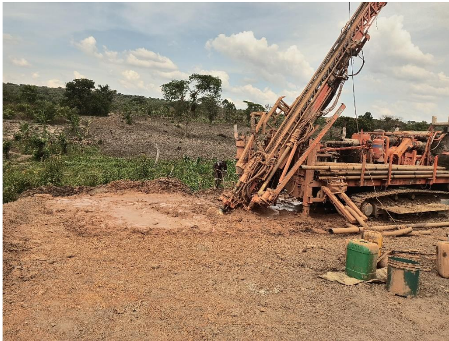
Figure 3: RC DDKNE 004 pre-collar installation at HEM 2 - Kabanga North-East
