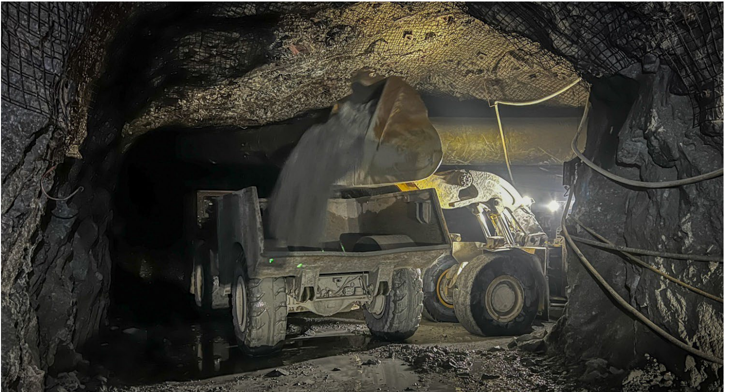
Figure 3 Komatsu underground loader, loading material into Komatsu 16 tonne underground truck
