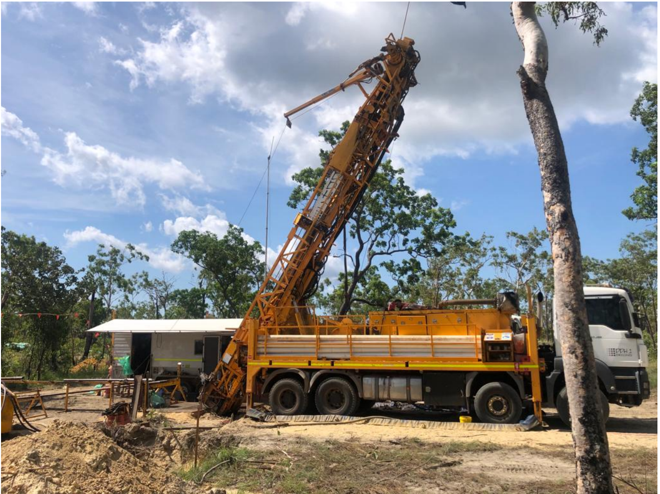
Figure 1. Showing the DDH1 Rig that will perform the deep diamond drilling at Lei Prospect
