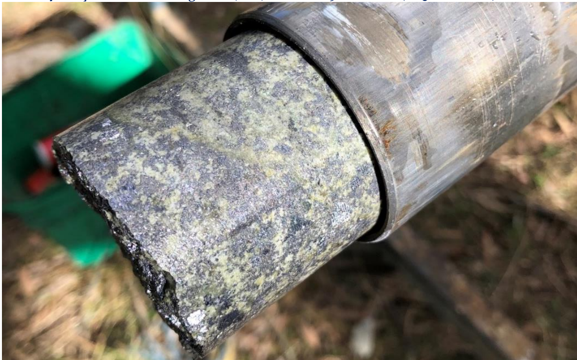
Photo 4: Very coarse blebs of galena (PbS) in WCS019 drill core (NQ 2 core size)
