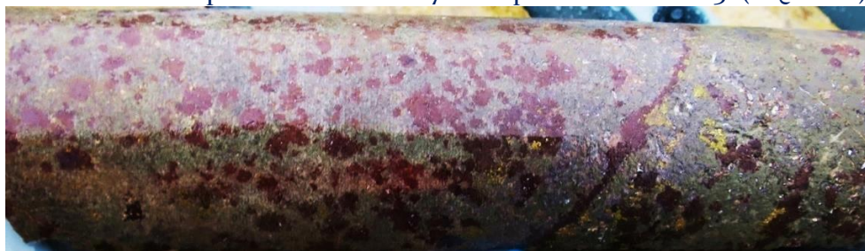
Photo 2: Coarse sphalerite blebs at 107.1m depth in hole WCS031 (NQ2 core)
