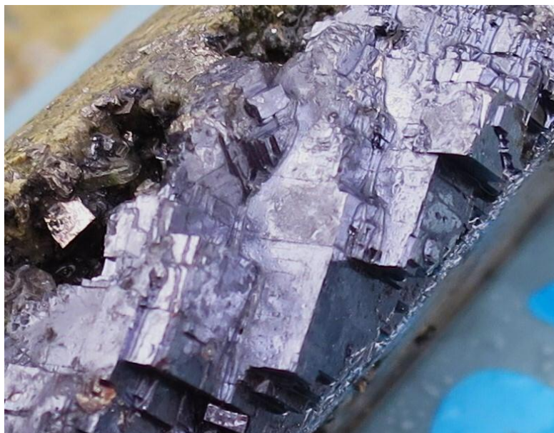
Photo 2: Coarse sphalerite blebs at 107.1m depth in hole WCS031 (NQ2 core)
